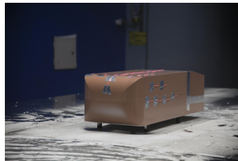
Figure 4.16: Tufts on Ahmed body with slant angle 10^\circ subjected to wind speed in the wind tunnel
