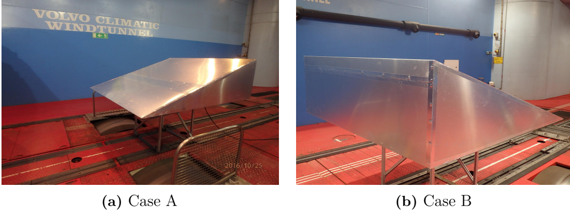
Figure 3.1: Wedge set-up in the climatic wind tunnel. Case A refers to the slant face facing the fan of the wind tunnel and Case B refers to the back face facing the fan of the wind tunnel.
