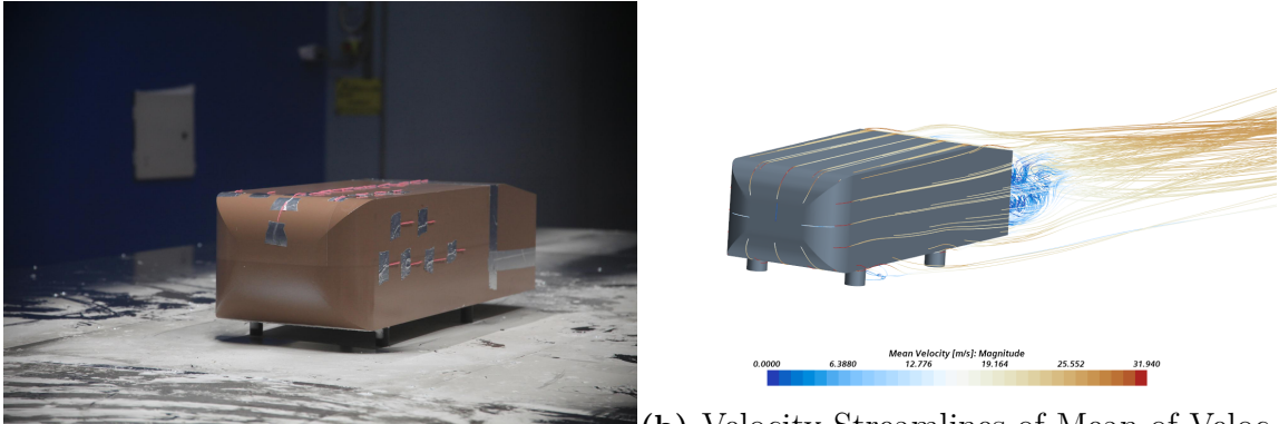
(a) Tufts on Ahmed body subjected to wind speed in the wind tunnel (b) Velocity Streamlines of Mean of Velocity: magnitude
