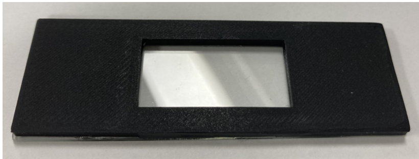
Figure 4.3: A 2.5 mm deep PLA mold glued to a microscopy glass slide.
