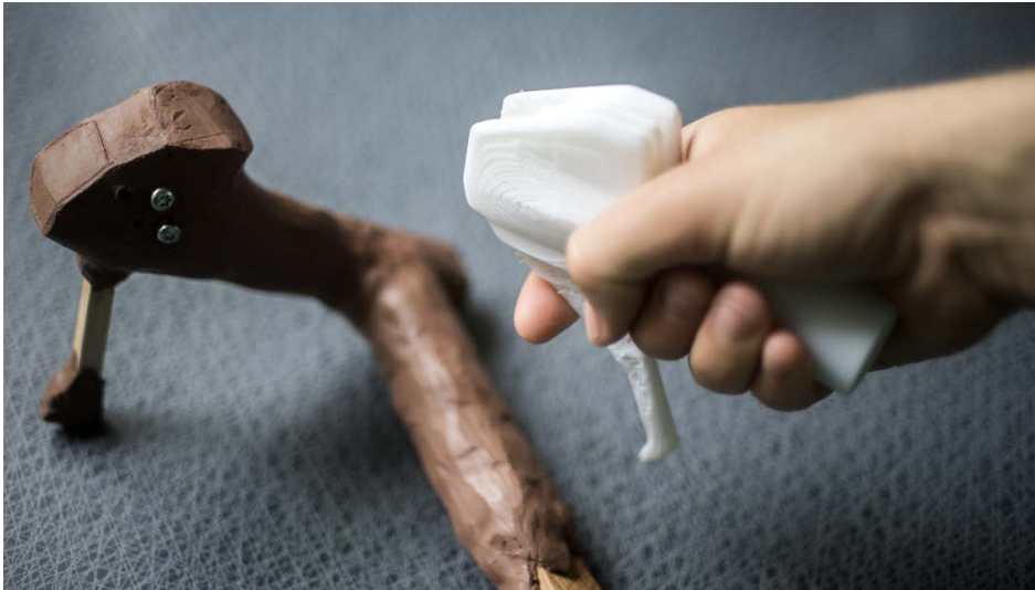
Figure 44: Mockup model and 3D print of handlebar ends.
