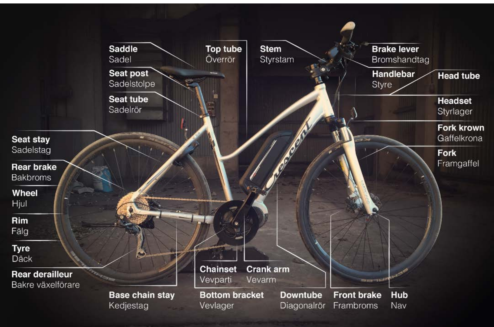
Figure 12: An illustration presenting the most essential bicycle components.
