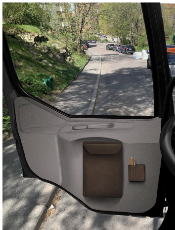
Figure 5: Picture of the driver side door with the paper and pen storage
