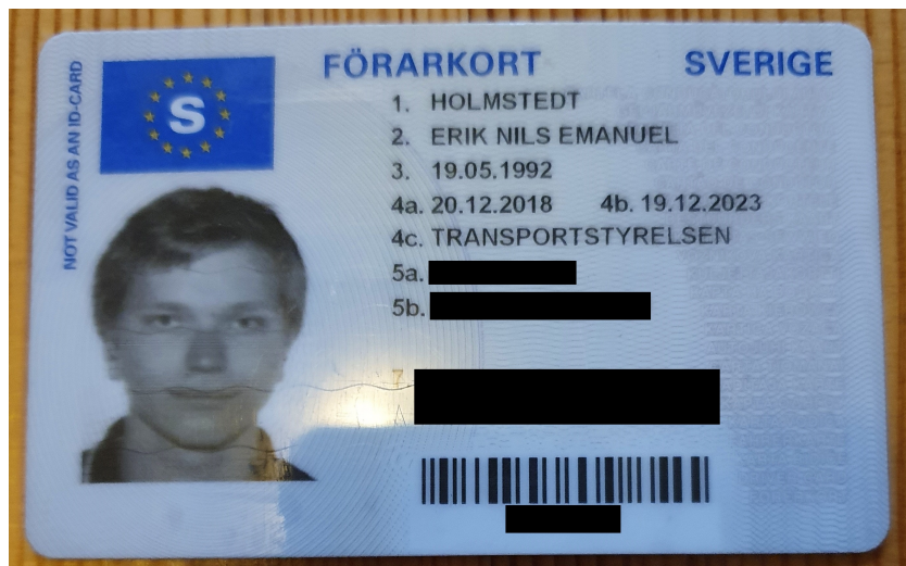
Figure 3.5: Picture of a Swedish driver card. The driver card is inserted into the Digital Tachograph to have drive and rest time data logged for the driver. Driver card information can be used for logging purposes to identify different drivers of a truck.
