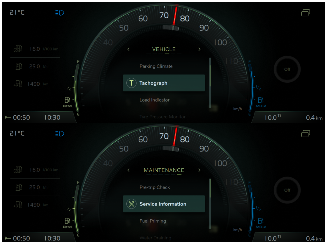
Figure 3.13: Picture of the menu in the Instrument Cluster. Seen here is two of the main headers: Vehicle and Maintenance. The user can navigate between the headers with the left and right buttons and scroll up and down under a header with the up and down buttons.
