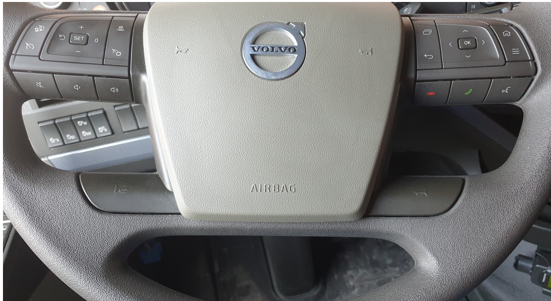
Figure 3.3: Picture of the steering wheel switches (SWS) in a Volvo Truck. On the left hand side buttons connected to CC/ACC functionality and volume control are placed. On the right hand side are buttons for navigation inside the HMI and phone functionality.
