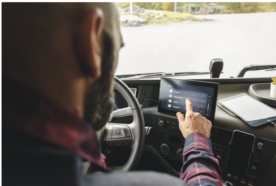
Figure 3.2: Picture of the Secondary Information Display. The display has touch functionality, but can also be controlled by the steering wheel switch buttons.
