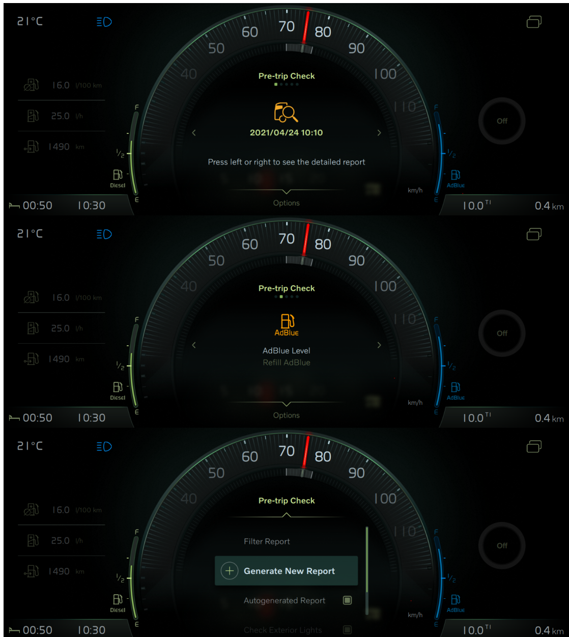
Figure 3.14: The views found in the Pre-Trip Inspection application in the Instrument Cluster. When entering the application a summary of the latest generated report is displayed, see in the upper picture. By scrolling left or right the driver can get more details on the issues identified by the function as seen in the middle picture. In the bottom picture the Options view for Pre-Trip Inspection is seen.
