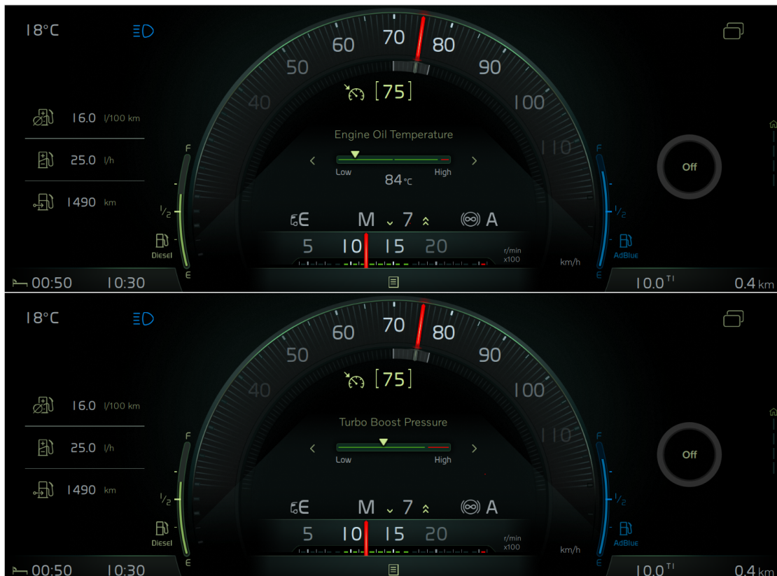
Figure 3.12: Example of two of the gauges available in the Instrument Cluster. In the upper picture the Engine Oil Temperature Gauge can be seen inside the speedometer and in the picture below the Turbo Boost Pressure Gauge can be seen. In total there are up to 17 different gauges available in the HMI, depending on the configuration of the truck.
