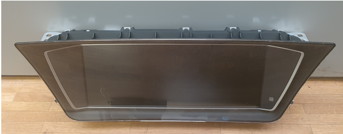
Figure 3.1: The hardware of the Instrument Cluster developed by Volvo Trucks that will be used for logging of user interaction in the thesis.
