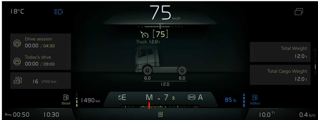
Figure 3.10: Picture of the Load Indicator Instrument View taken in HMI simulation tool.
