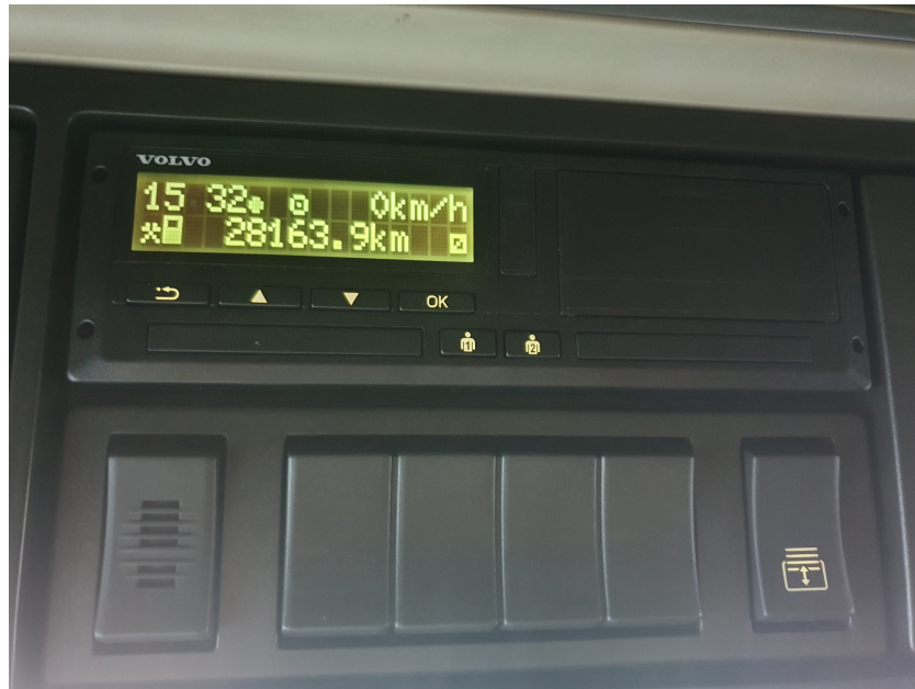
Figure 3.4: Picture of a Digital Tachograph. The driver card is inserted into the card holder to have drive time data logged for the driver. The tachograph has two card slots: the first slot is for the driver and slot two is to be used by a co-driver.
