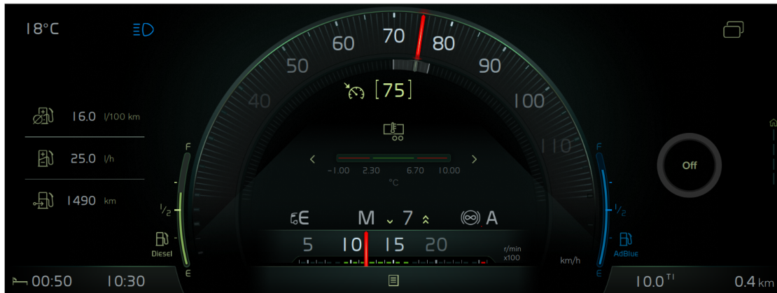
Figure 3.8: Picture of the Analog Instrument View taken in HMI simulation tool. The Analog View is meant to be reminiscent of a classic mechanical Instrument Cluster with an analog gauge.
