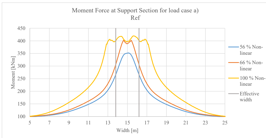
Figure 5.28: Moment distribution for case Ref subjected to load case a). Utilization ratio of maximum load capacity in non-linear analysis. The effective width used in linear analysis is presented.
