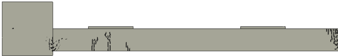
(a) The most significant cracks per element with a crack width size over 0.15 mm.
