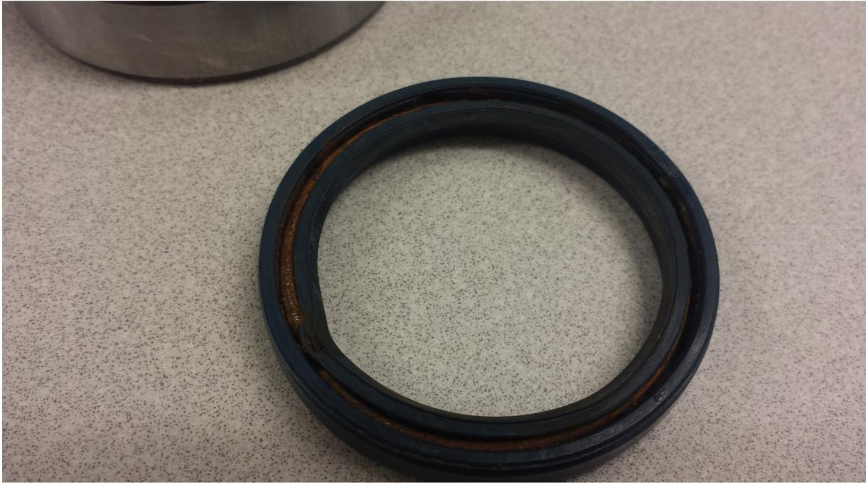
*Figure 9.1 Corrosion in the Couette cell.*
