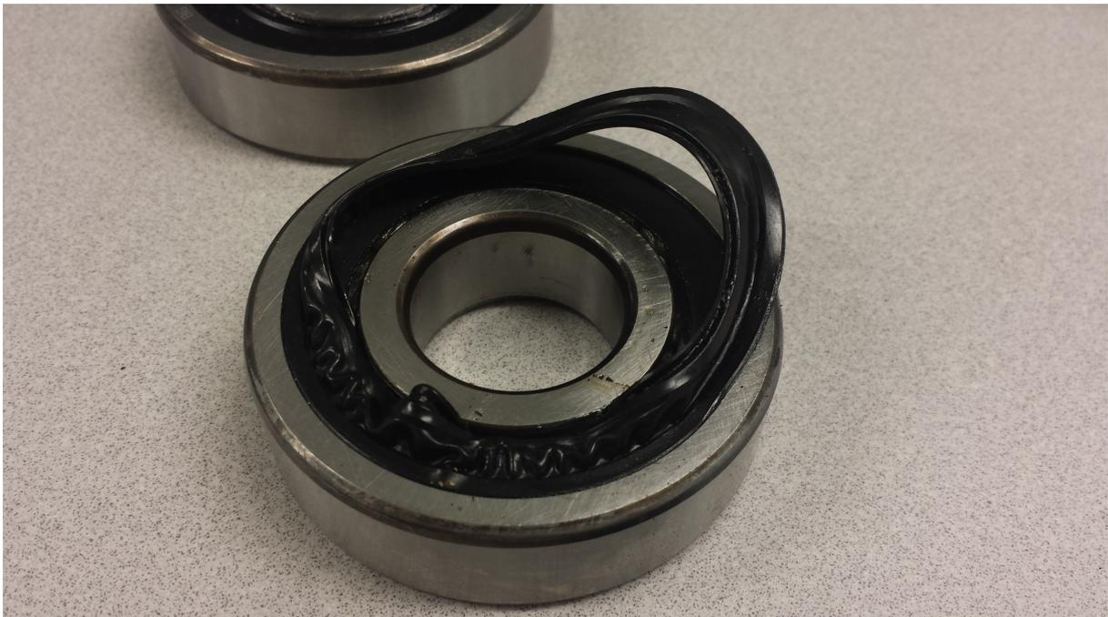
*Figure 9.2 Stretched rubber due to contact with benzyl alcohol.*
