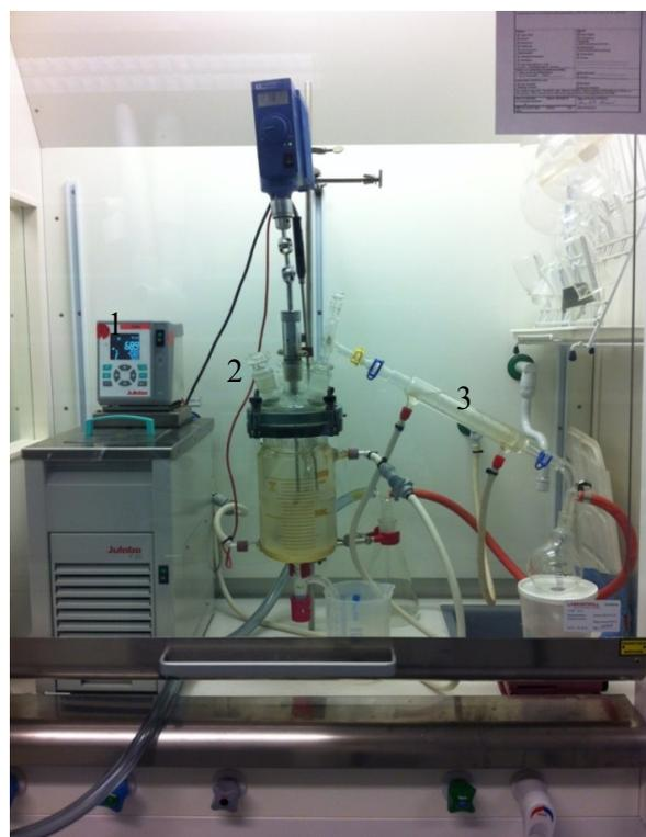
*Figure 3.1 Experimental setup for the ESE-process containing refrigerated and heating circulator (1), double-walled reactor (2) and condenser system (3).*
