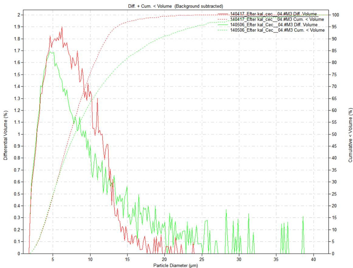
Figure 4.28 Particle size distributions from Coulter counter for syntheses with and without thickener of the organic phase, while at the same time using the Couette cell. The green curve represents 5 wt% addition of poly(isobutyl methacrylate) and the red curve is the reference system with no thickener.
