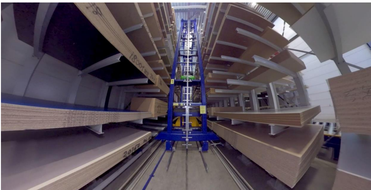
Figure 4.14: A high-bay storage and picking solution of sheet materials from Systraplan.
