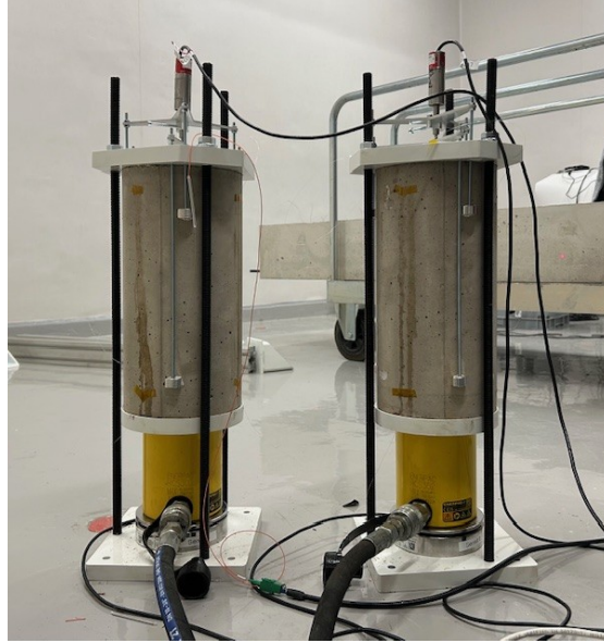
Figure 3.8: Cylinder experiment measuring total strain from creep and shrinkage.
