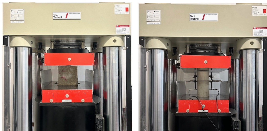
Figure 3.7: a) Compressive strength cube test. b) Modulus of elasticity cylindrical test. Both tests were performed in a Toni Technik machine.
