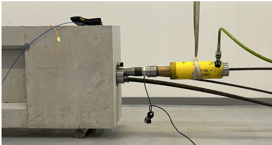
Figure 3.6: Post-tensioning system and hydraulic jack.
