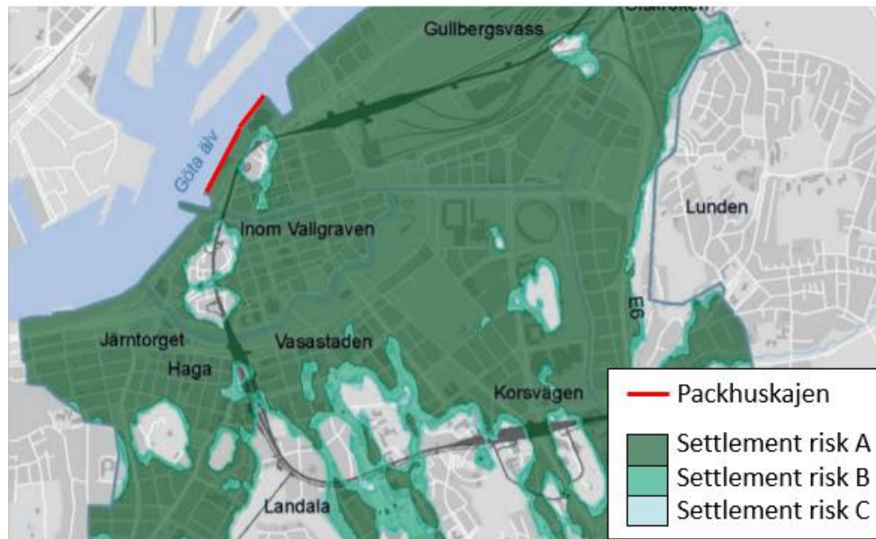
Figure 13: Risk areas for settlement sensitive clay. Settlement risk A represents the area that shows the most probable distribution of > 1 meter settlement sensitive clay. B and C represent areas with relatively high probabilities of settlement sensitive clay > 1 meter. Outside the marked areas, the probability of the presence of settlement sensitive clay > 1 meter is very low (modified from STA, 2016b).
