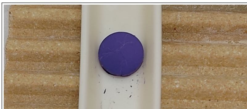
Figure 5.1: Pellet after being annealed at 1400 °C for 6 hours and air quenched, demonstrating the purple colour it obtains.
