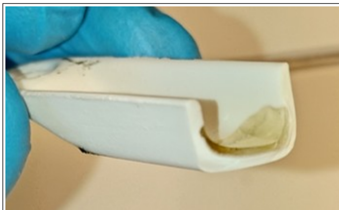
Figure 5.2: Melted pellet in an alumina boat after being heated at 1500 °C for 5 h. This procedure also had the side effect of breaking the alumina boat.
