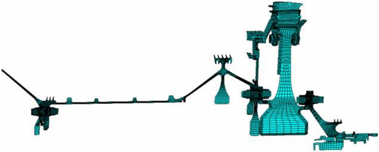
Figure 3.3: The 2D/3D hybrid model of the HPT.
