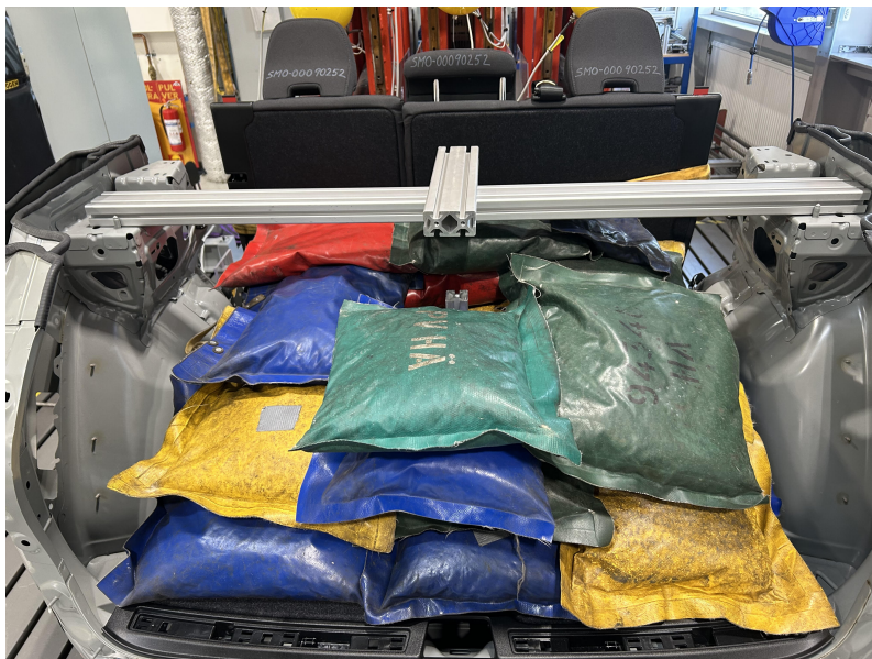
Figure 4.5: Upper limit load test setup with uniformly distributed load on the load floor
