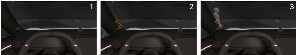
Figure 8.5: Sequence of Light that Illuminates When an Object is Detected
