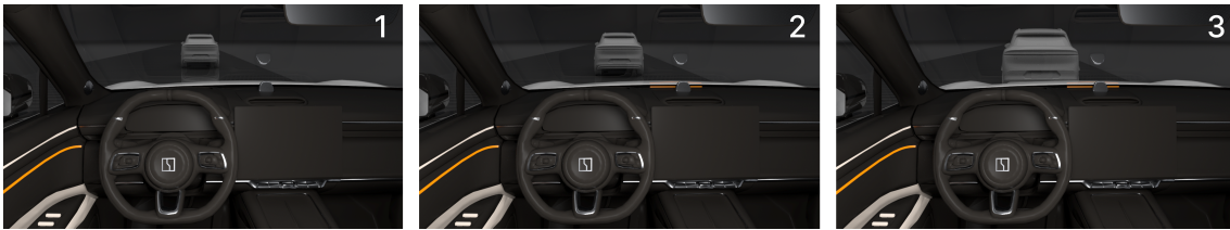
Figure 8.9: Sequence of Light That Illuminate When Tailgating
