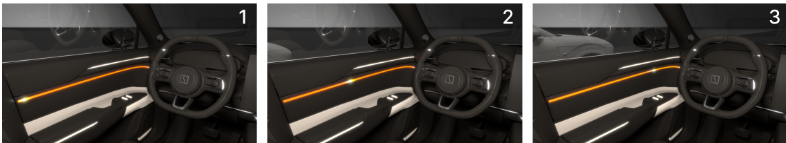
Figure 0.2: Three Sections of Moving Ambient Lights on Front Door
