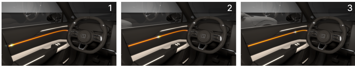
Figure 2.2: Three Sections of Moving Ambient Lights on Front Door
