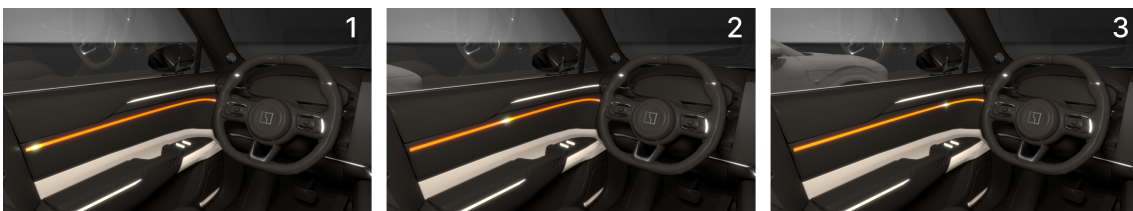
Figure 8.3: Sequence of a Sweeping Pulse Representing a Car Doing an Overtake
