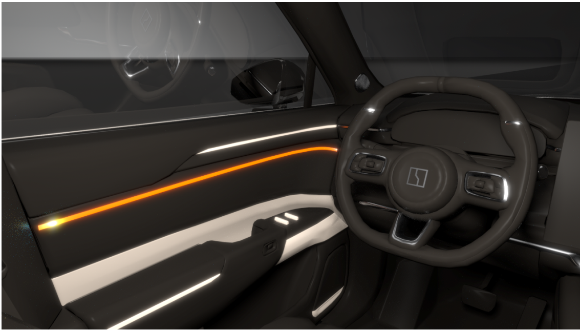
Figure 8.2: Ambient Light Source on Front Door
