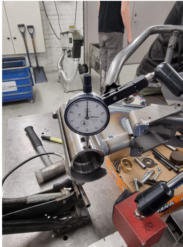
Figure 3.18: Placement of dial indicator for lateral test
