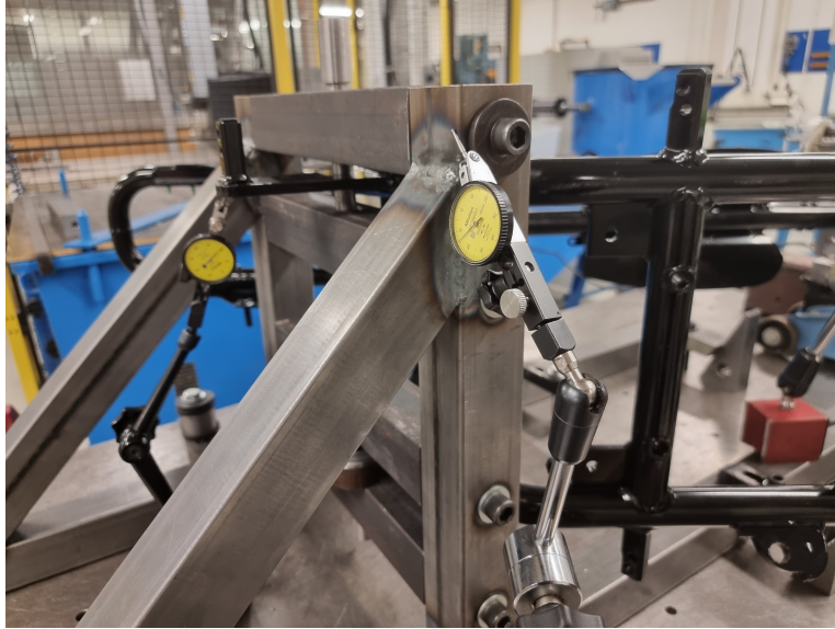
Figure 3.15: Placement of dial indicator for test rig flex measurement
