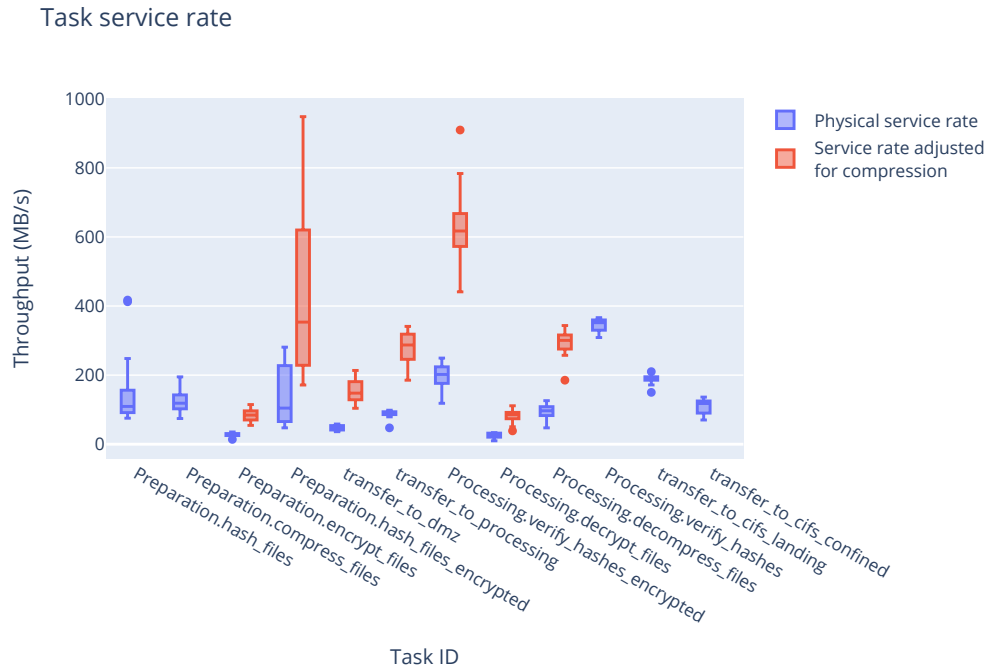
Figure 6.5: The service rate of each task, i.e. the rate at which it processes its input, is shown in blue. For tasks operating on compressed data (all tasks from Preparation.compress_files until Processing.decompress_files ), the effective service rate over raw data is shown in red. Notably, the transfer_to_dmz now reaches an effective rate of over 150 MB/s over the bottleneck link.
