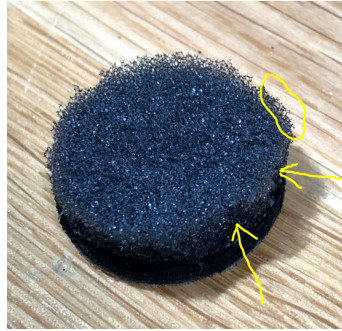
Figure 3.11: Foam damaged around the circumference.
