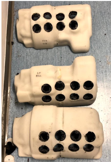
Figure 3.33: Encapsulation of Special Sample 1 - 90% Coverage.
