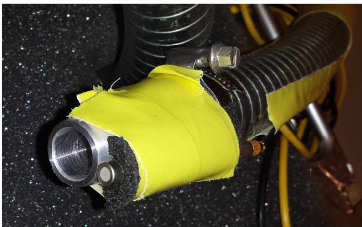
Figure 3.40: Hose Pipe, Microphone position and nozzle details
