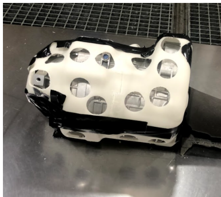
Figure 3.36: Encapsulation of Carrier - 85% Coverage.
