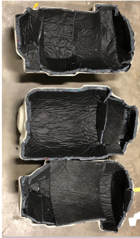
Figure 3.27: Encapsulation of Sample 30 - 100% Coverage.
