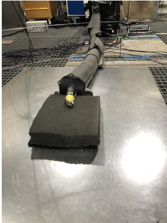
Figure 3.42: 3 layer Covering on the hose pipe 10 mm Foam + 2mm Mass Layer + 10 mm Foam
