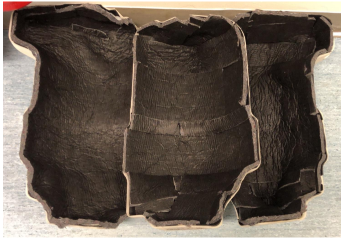
Figure 3.24: Encapsulation of Sample 24 - 100% Coverage.
