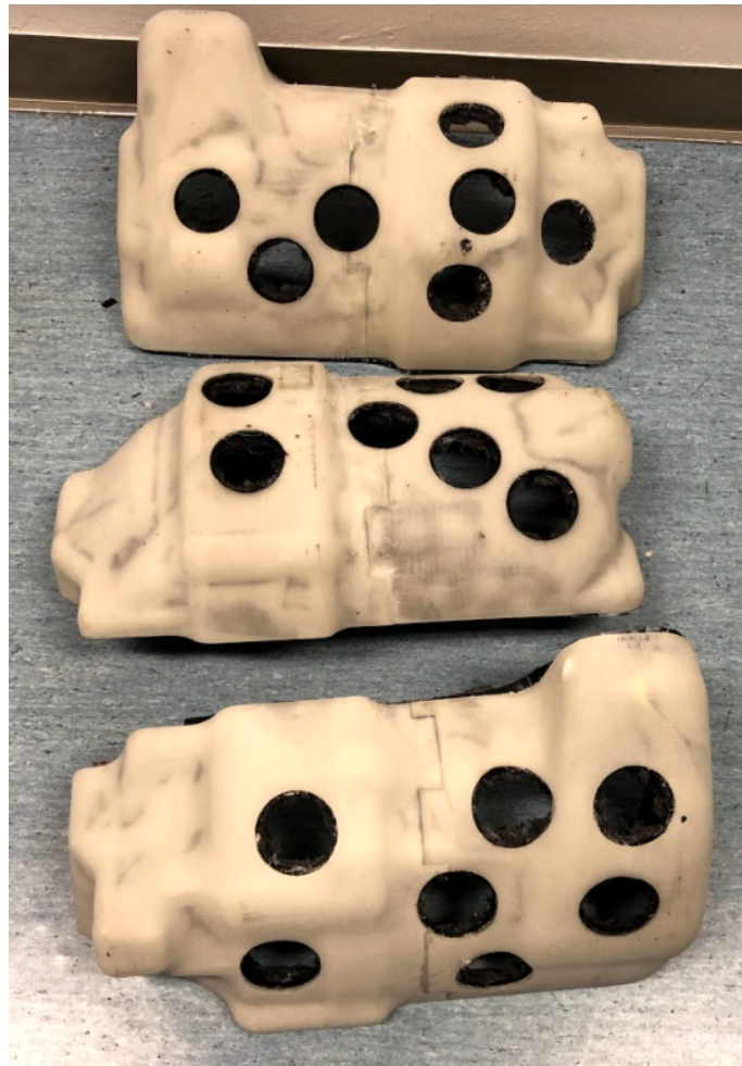
Figure 3.26: Encapsulation of Sample 24 - 90% Coverage.
