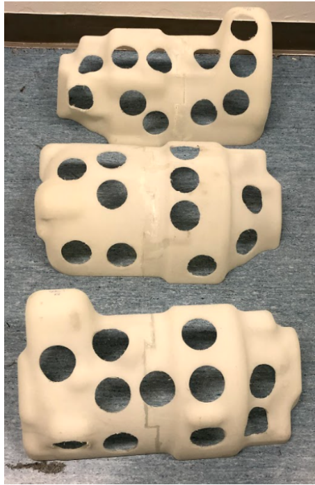
Figure 3.35: Encapsulation of Carrier - 90% Coverage.
