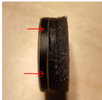
Figure 3.10: Rubber tape wrapped around the carrier.
