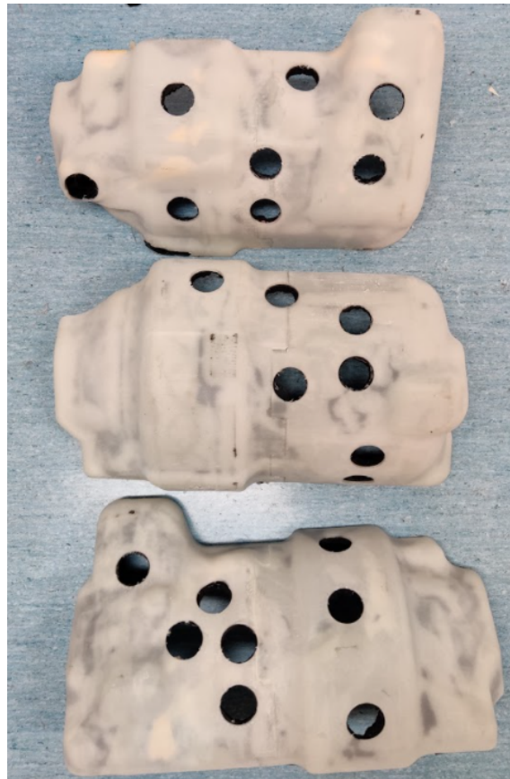
Figure 3.21: Encapsulation of Sample 17 - 95% Coverage.
