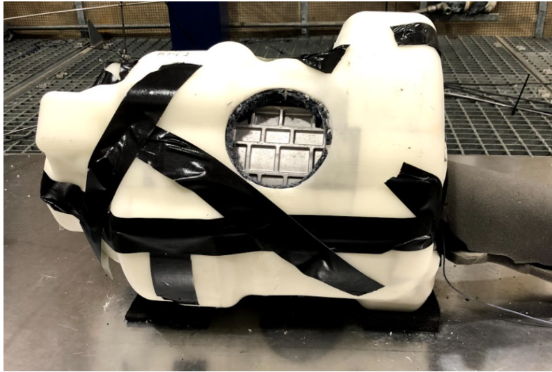
Figure 3.28: Encapsulation of Sample 30 - 95% Coverage.
