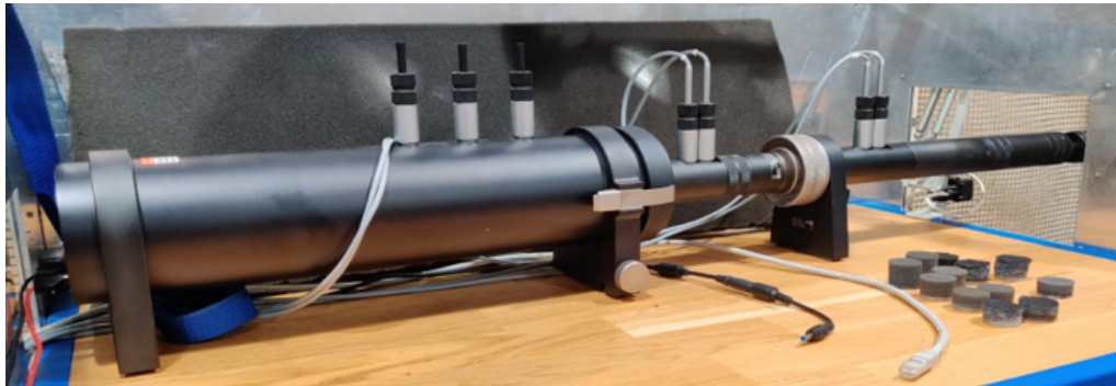
Figure 3.5: B&K Pulse - Impedance Tube Setup at Volvo Cars' Facility.
