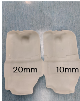
Figure 3.18: Carrier Templates - 10 mm and 20 mm Offset.
