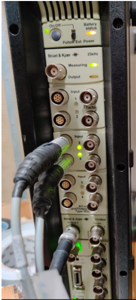
Figure 3.6: B&K Acoustic Material Test Front-end.
