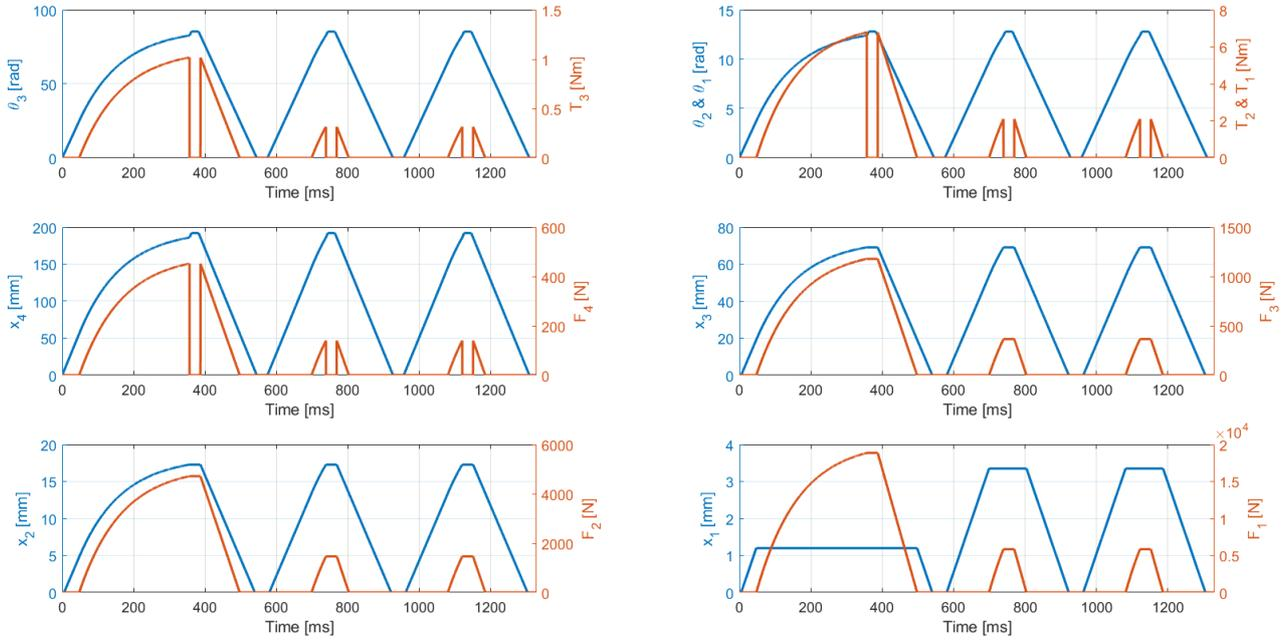
Figure A.1: Force and displacement simulation of a normally open clutch system without wear compensation.
