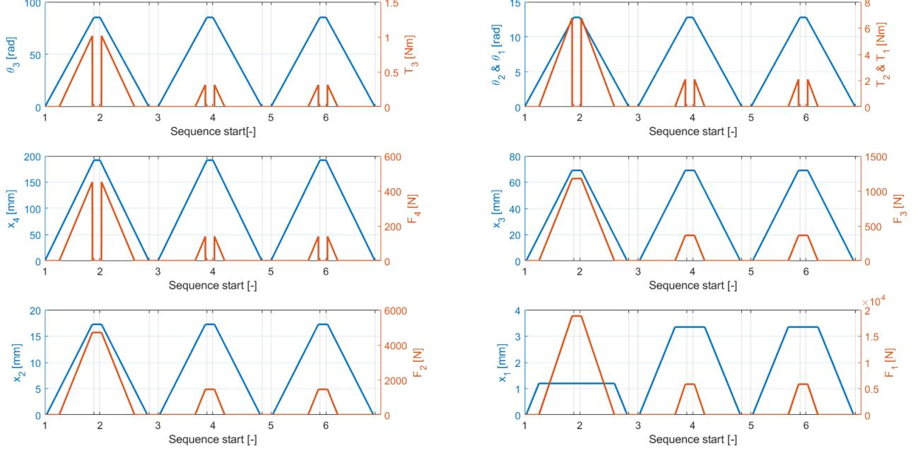
Figure 3.36: Force and displacement, time independent simulation of a normally open clutch system without wear compensation.
