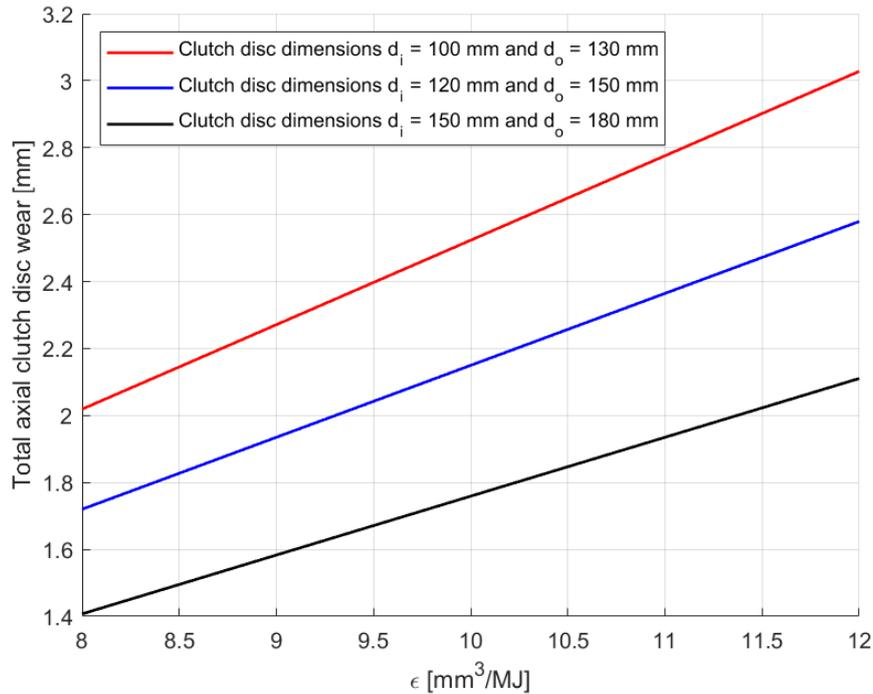
Figure 3.27: Illustration of axial clutch wear during a complete life cycle.
