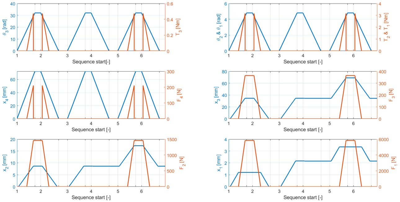
Figure A.8: Force and displacement, time independent simulation of a normally open clutch system with wear compensation near actuator.
