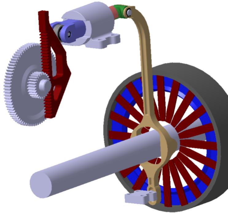
Figure 4.9: *Illustration of the wear compensation mechanism embedded into the actuation system.*
