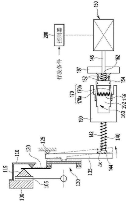
Figure 3.6: Schematic of the step concept in an engaged clutch position.
