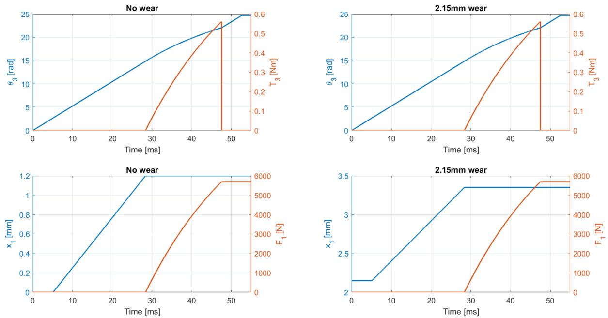
Figure B.5: Clutch actuation performance with a ramp pitch angle of  $35^\circ$  and displacement compensation.
