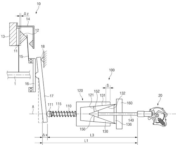
Figure 3.11: Schematics of the wedge concept in an engaged position with a worn clutch.
