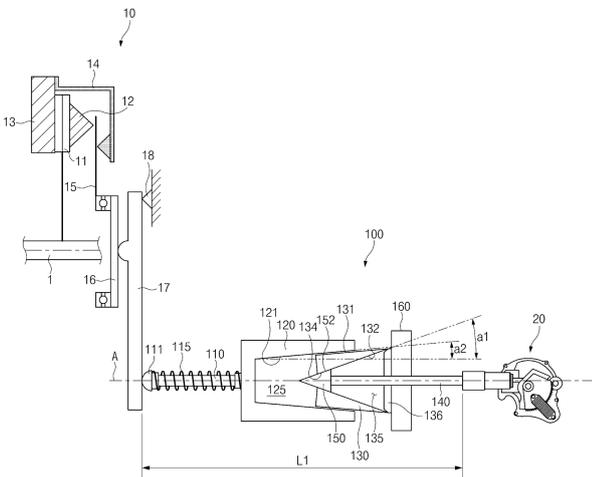
Figure 3.9: Schematics of the wedge concept in an engaged clutch position with an unworn clutch.
