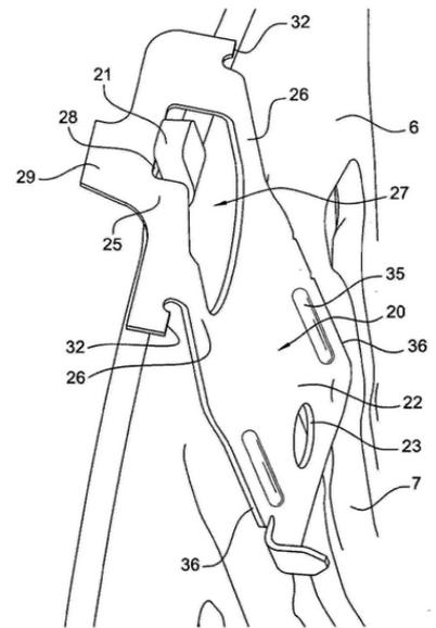
Figure 3.19: Schematic of the pawl and the tooth.
