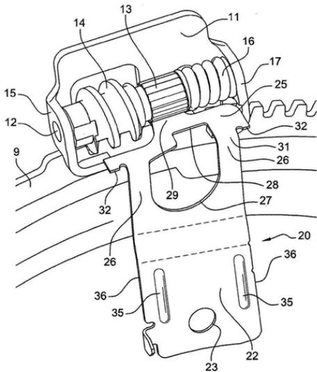
Figure 3.18: Schematic of the pawl concept and the worm gear.
