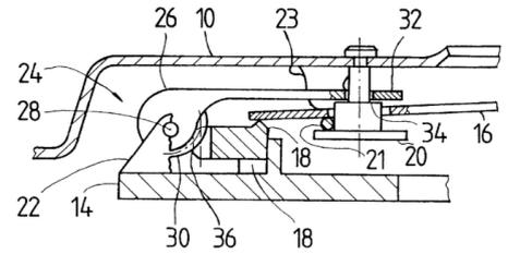
Figure 3.21: Schematic of the lever concept when the clutch is engaged.
