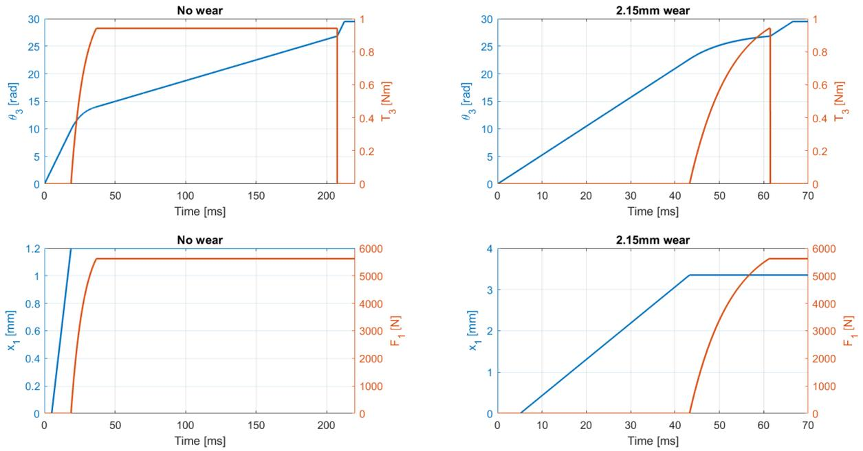
Figure B.4: Clutch actuation performance with a ramp pitch angle of  $50^\circ$  and force compensation.
