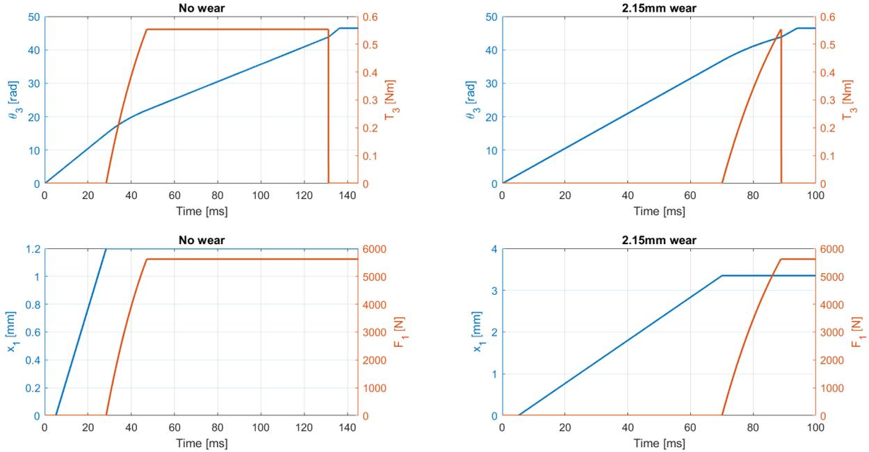
Figure 4.2: *Clutch actuation performance with force compensation.*
