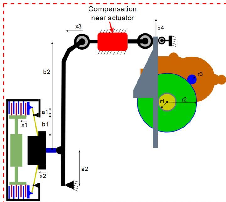
Figure 3.32: *Schematics of compensation near actuator with a normally closed clutch.*
