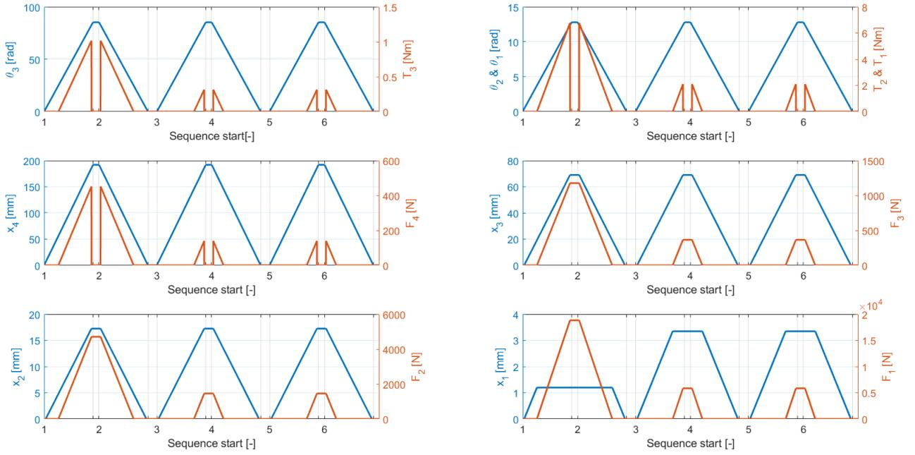
Figure A.2: Force and displacement, time independent simulation of a normally open clutch system without wear compensation.
