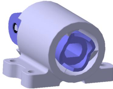
Figure 4.6: A close up of the sleeve inside the housing.
