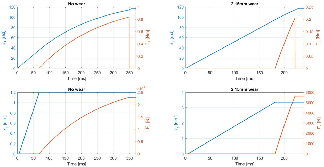
Figure B.1: Clutch actuation performance with a ramp pitch angle of  $14.5^\circ$  and no wear compensation
