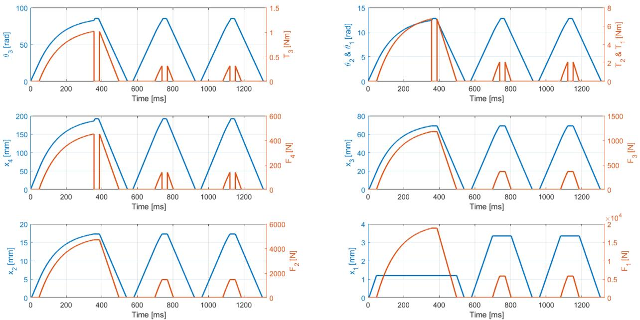
Figure 3.35: Force and displacement simulation of a normally open clutch system without wear compensation.
