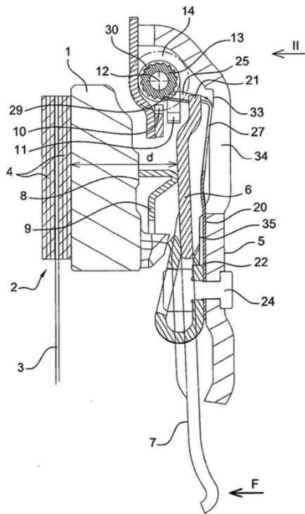
Figure 3.16: Schematic overview of the pawl concept.
