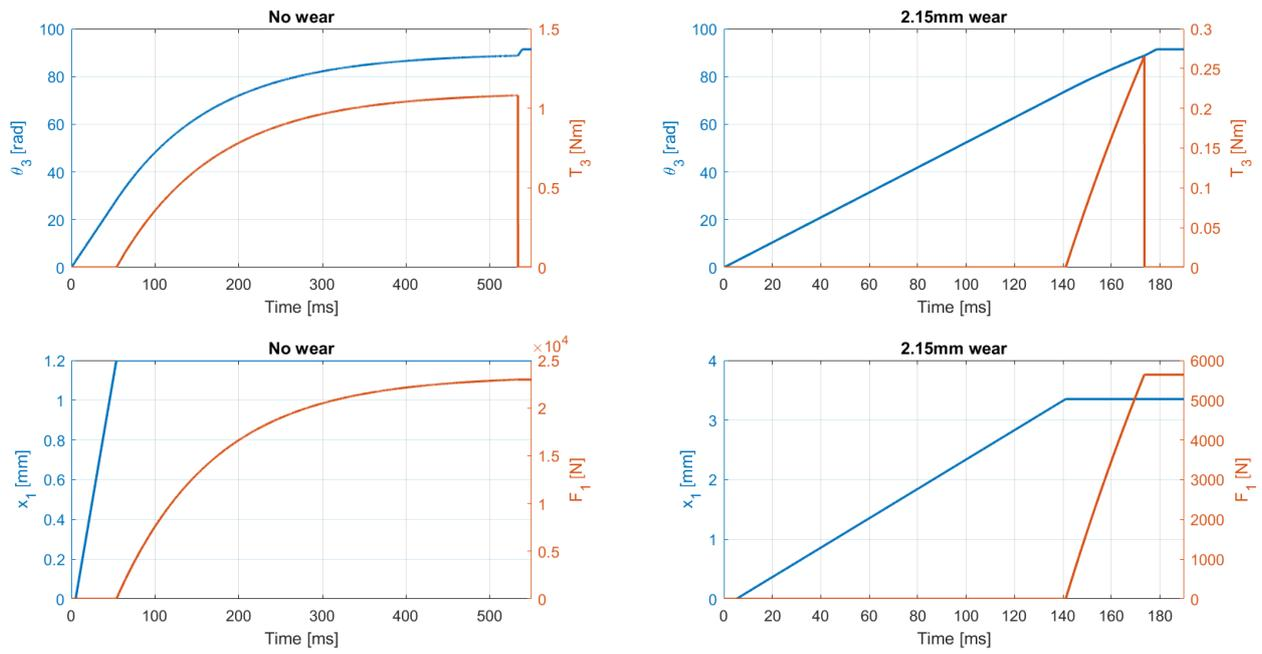
Figure B.2: Clutch actuation performance with a ramp pitch angle of  $18.5^\circ$  and no wear compensation.
