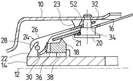
Figure 3.22: Schematic of the lever concept when the clutch is engaged and wear occurs.
