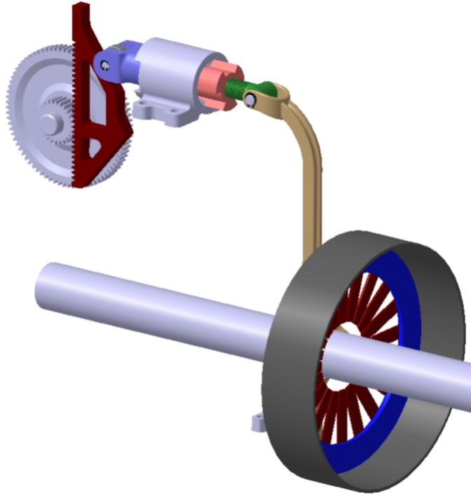
Figure 4.8: *Illustration of the wear compensation mechanism embedded into the actuation system.*
