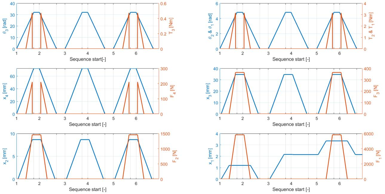
Figure A.6: Force and displacement, time independent simulation of a normally open clutch system with wear compensation near discs.
