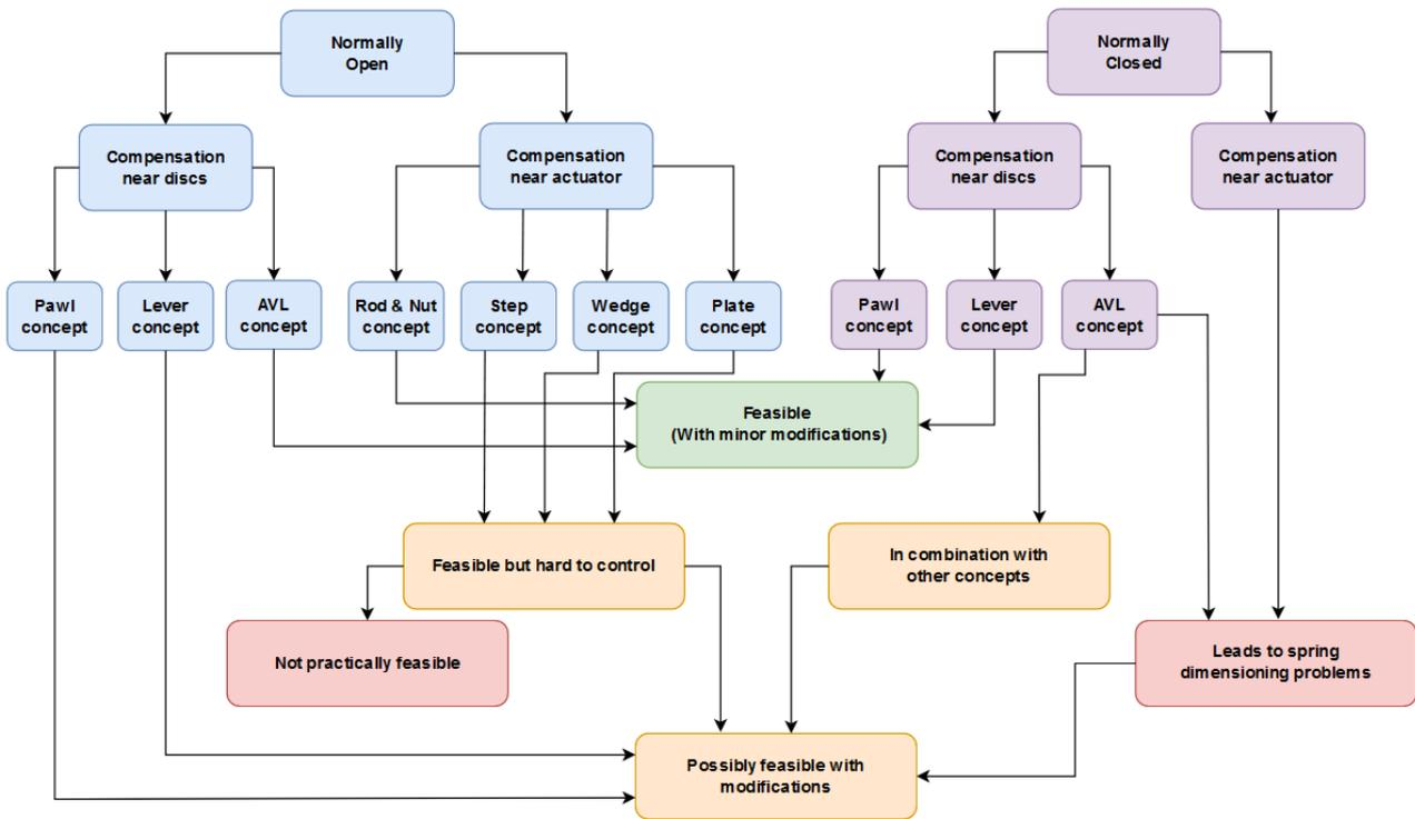
Figure 3.34: Tree showing the different concepts and if they will function in the system.
