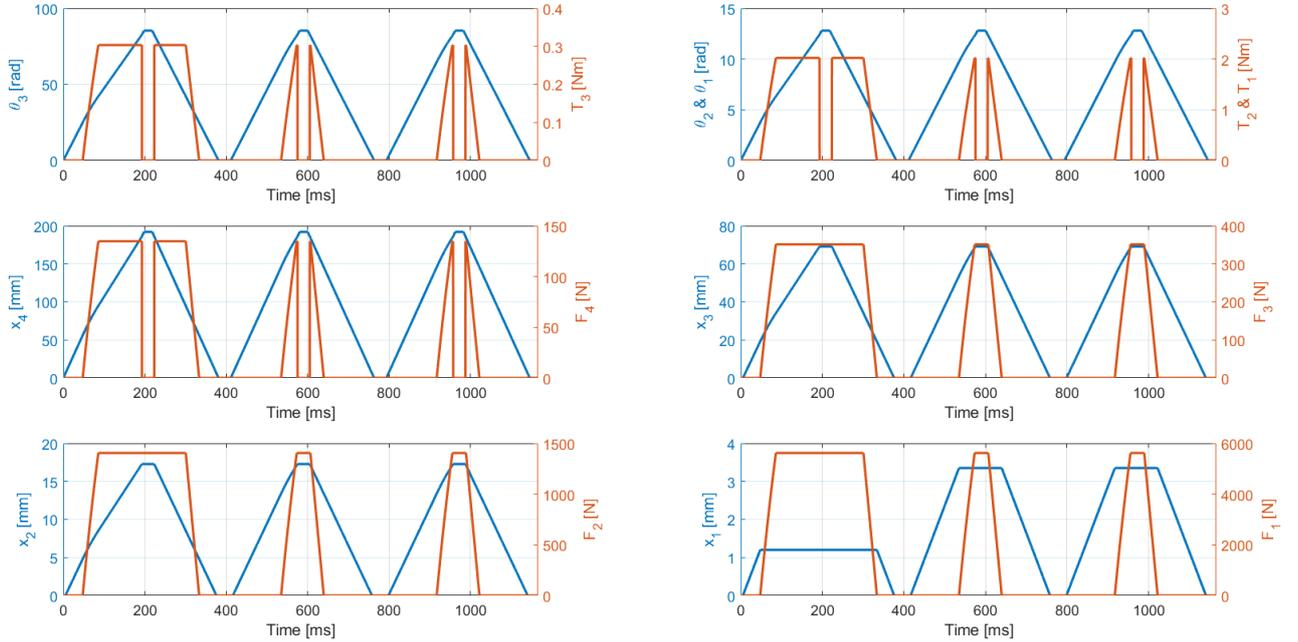
Figure A.3: Force and displacement simulation of a normally open clutch system with the AVL force limiter.
