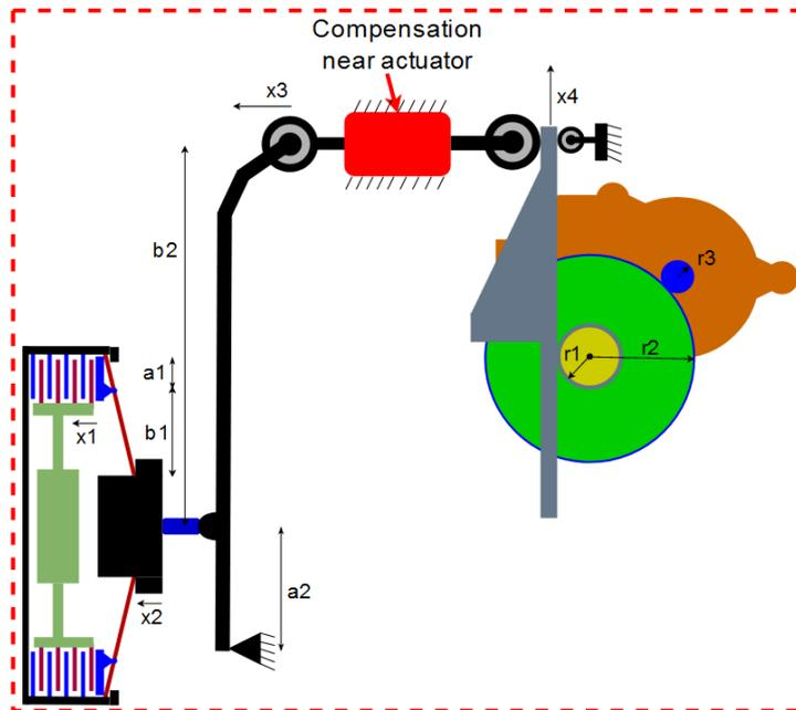
Figure 3.31: *Schematics of compensation near actuator with a normally open clutch.*
