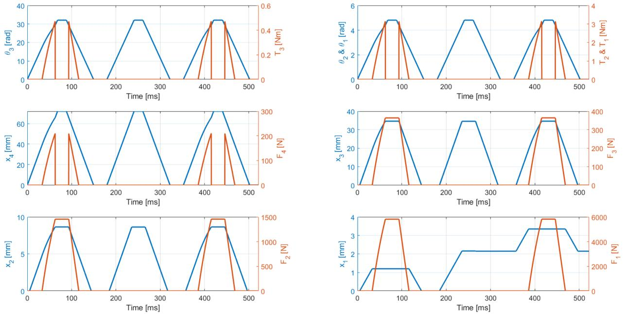
Figure A.5: Force and displacement simulation of a normally open clutch system with wear compensation near discs.
