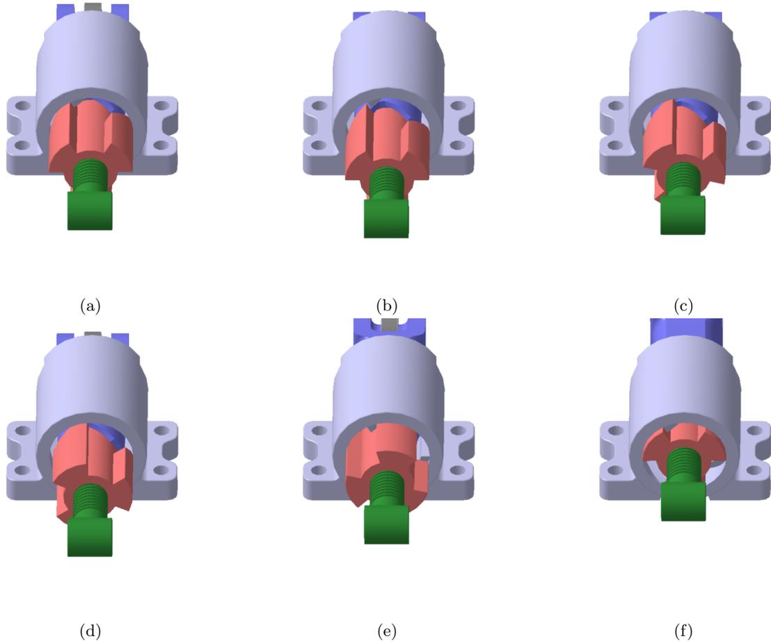
Figure 4.7: *Illustration of the wear compensation mechanism during a compensation.*
