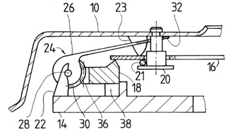
Figure 3.23: Schematic of the lever concept after the wear adjustment have occurred and the clutch is disengaged.
