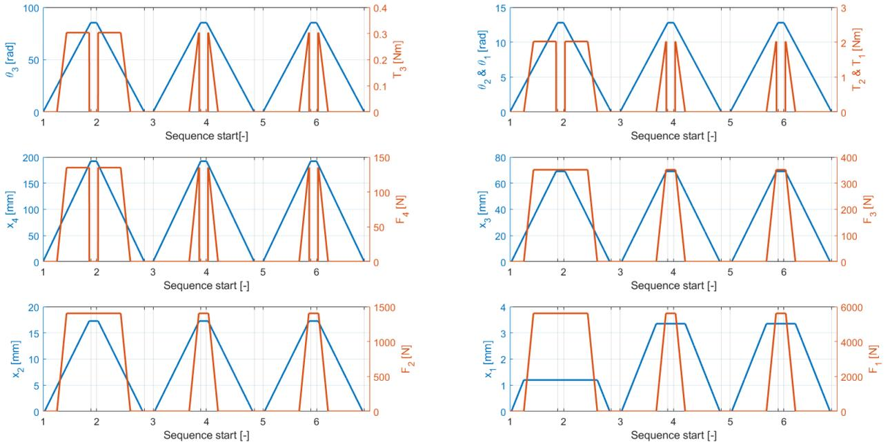
Figure A.4: Force and displacement, time independent simulation of a normally open clutch system with the AVL force limiter.
