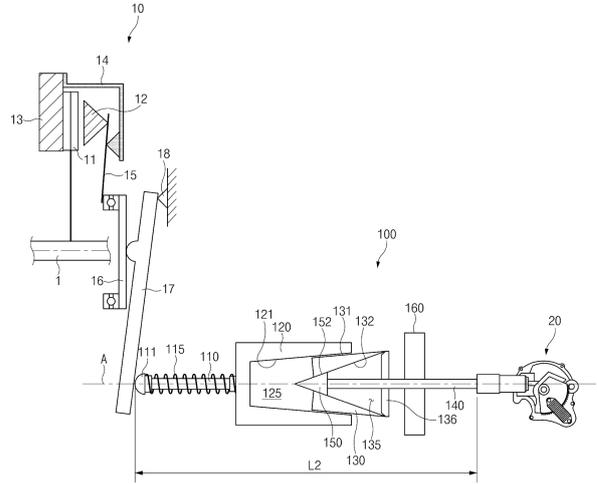
Figure 3.10: Schematics of the wedge concept in a disengaged position with an unworn clutch.
