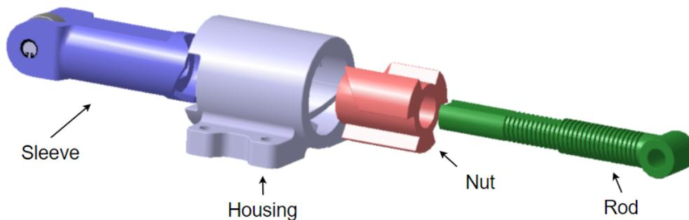
Figure 4.5: Exploded view of the wear compensation mechanism.
