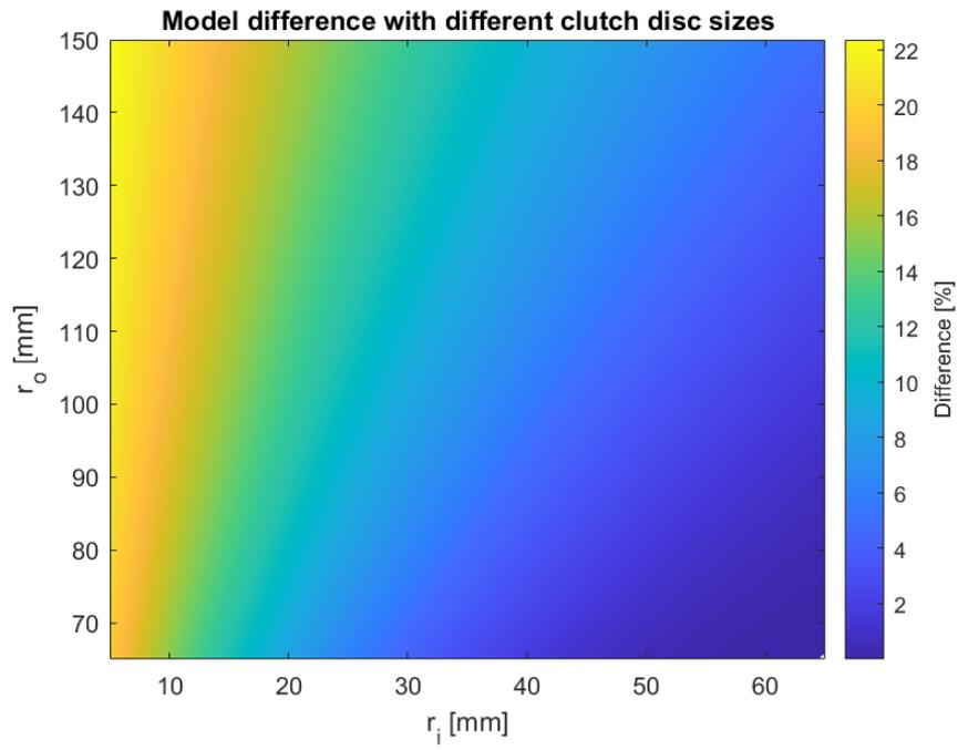
Figure 2.1: Illustration of how the unworn clutch model differ compared to the model for a used disc.
