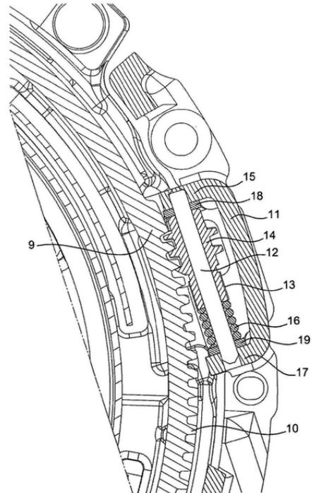
Figure 3.17: Schematic of the pawl concept and the worm gear.
