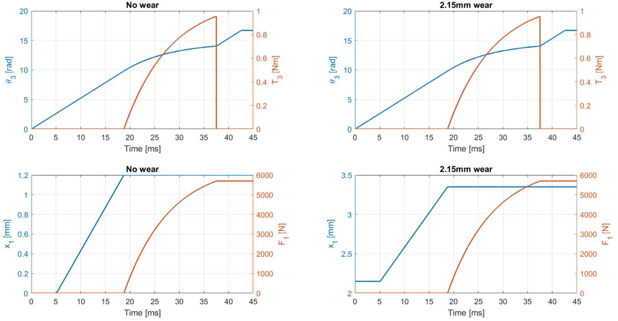
Figure B.6: Clutch actuation performance with a ramp pitch angle of  $50^\circ$  and displacement compensation.
