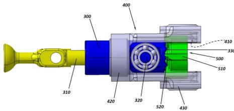
Figure 3.3: 3-D CAD of the threaded rod and nut concept. Side view with released actuation.
