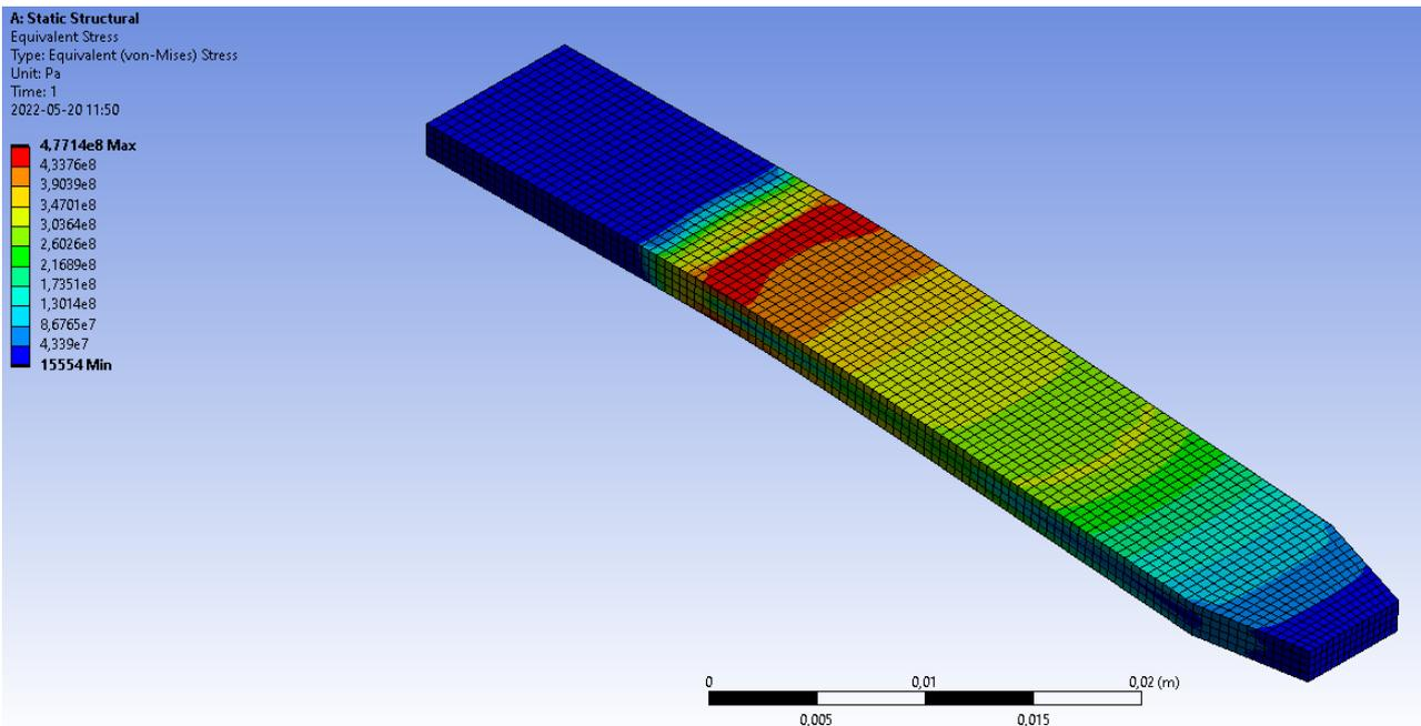
Figure 4.4: Ansys calculation on stress distribution over the pressure plate lever.
