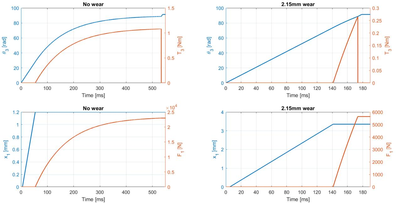
Figure 4.1: *Clutch actuation performance without wear compensation.*
