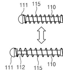
Figure 3.12: Schematics of the push rod assembly.
