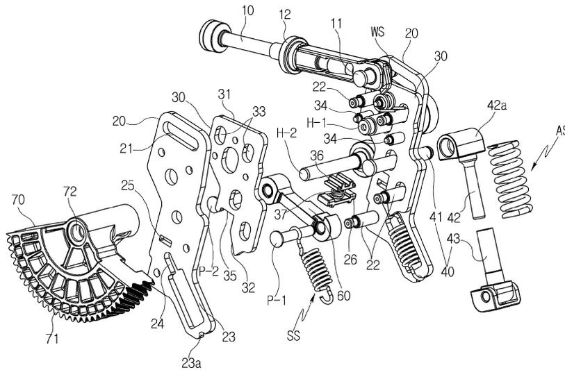
Figure 3.15: Exploded view schematics of the adjuster plate concept.
