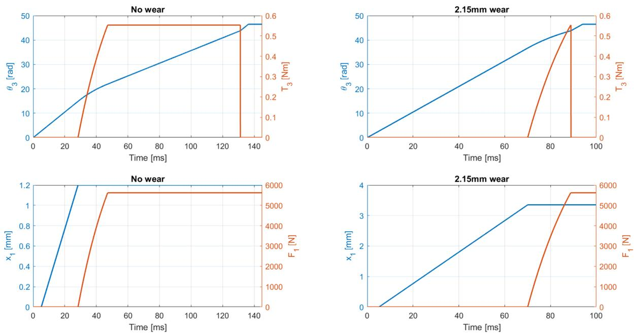
Figure B.3: Clutch actuation performance with a ramp pitch angle of  $35^\circ$  and force compensation.
