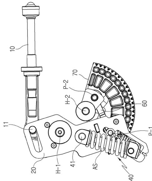
Figure 3.14: Schematics of the adjuster plate concept with the housing removed.
