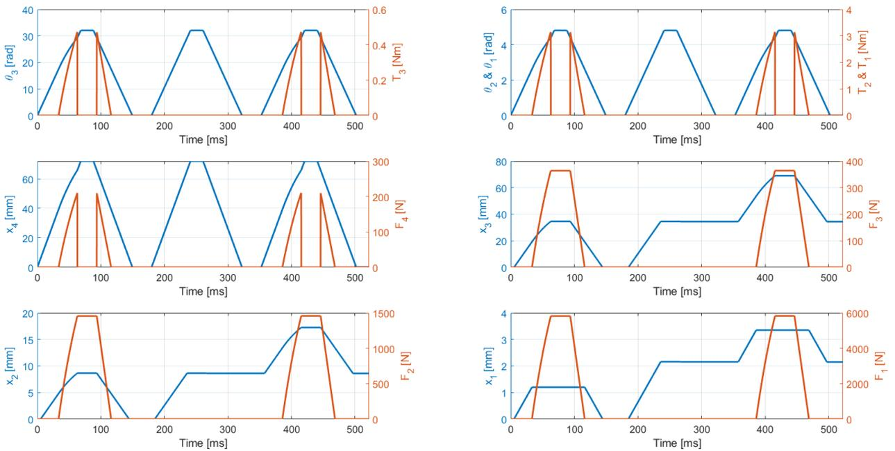
Figure A.7: Force and displacement simulation of a normally open clutch system with wear compensation near actuator.
