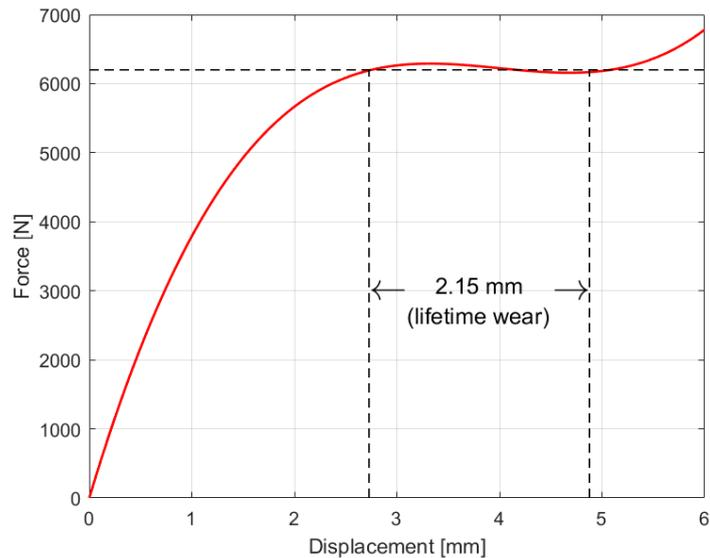
Figure 3.26: Force vs. displacement characteristics of an example diaphragm spring to be used as a force limiter.
