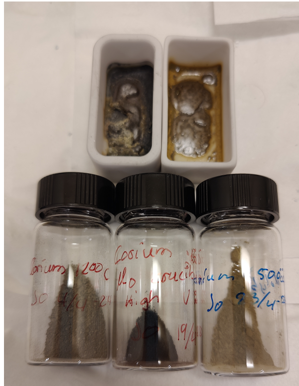
Figure 4.4: All samples of synthesized corium. Top row: Alumina crucible 1500°C. Left: Alumina crucible treated with calcium carbonate. Right: untreated crucible. Bottom row: Powdered Corium samples. From left to right: Standard corium in alumina crucible 1200°C, High U ratio in Mo crucible 1500°C, Regular corium in Mo crucible 1500°C.
