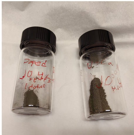
(a) Samples of the doped \text{UO}_2 and the sample of \text{UO}_2 + \text{CaO} heated to 1200^\circ\text{C} .
