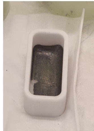
(b) Alumina crucible with the coating of \text{CaO} and \text{UO}_2 after heating to 1500^\circ\text{C} .
