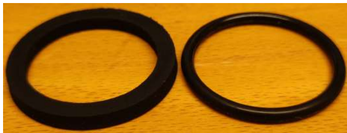
Figure A.11: Visualization of square rubber seal as compared to the round rubber seal
