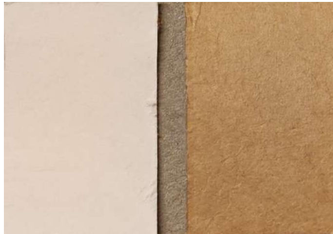
Figure 5.3: Visualisation of sample paperboard's top and bottom faces due to its double layered construction (Material B pictured here)
