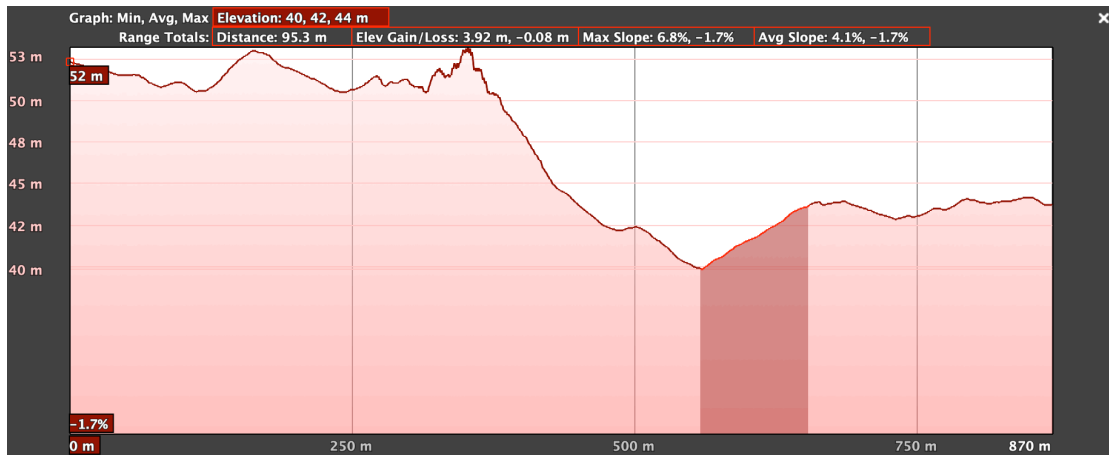
Figure B.13 The elevation profile for the e-scooter route Kvarnstensvägen 8 to Kvarnfallsvägen, where the second inclination is marked.
