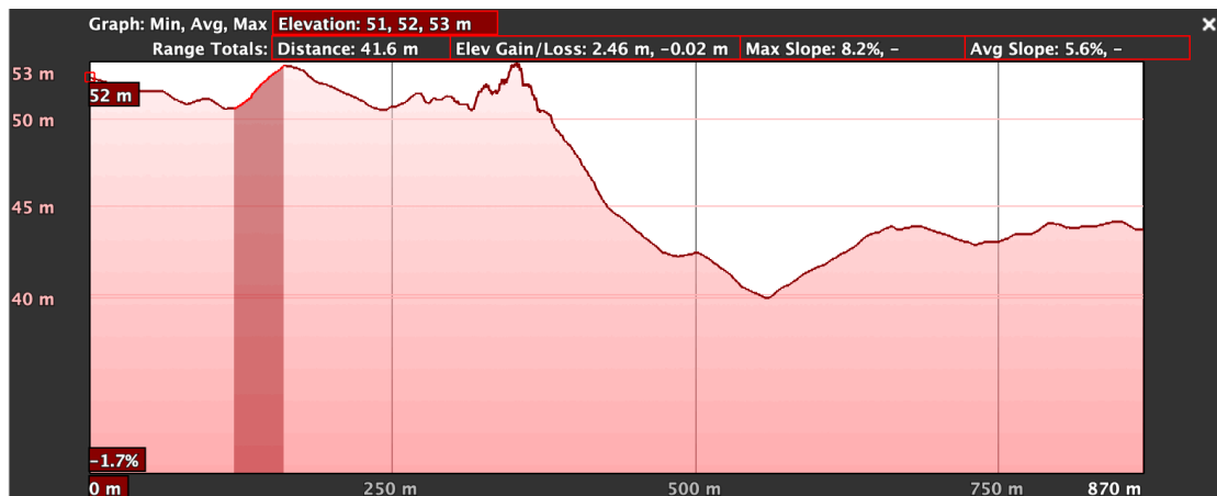
Figure B.12 The elevation profile for the e-scooter route Kvarnstensvägen 8 to Kvarnfallsvägen, where the first inclination is marked.
