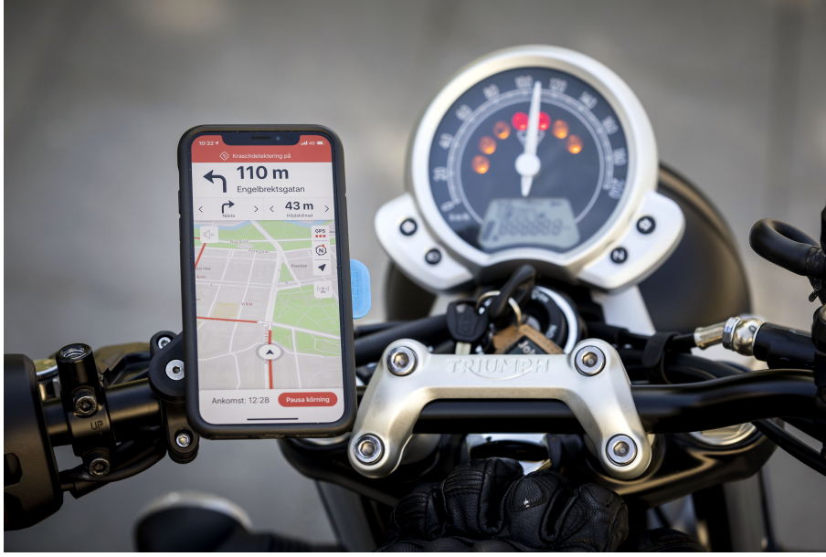
Figure 3.2: Recommended configuration of the smartphone mounting. Source: Detecht.
