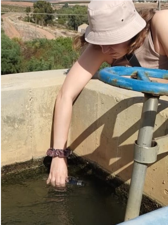
Figure 3.13: Sampling of raw water at Piketberg DWTP.
