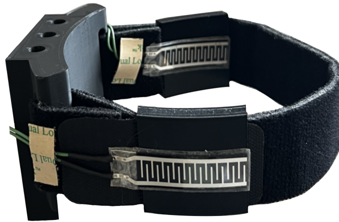
Figure 3.13: The 3D-printed sensor supports attached to the Velcro, including tactile sensors.
