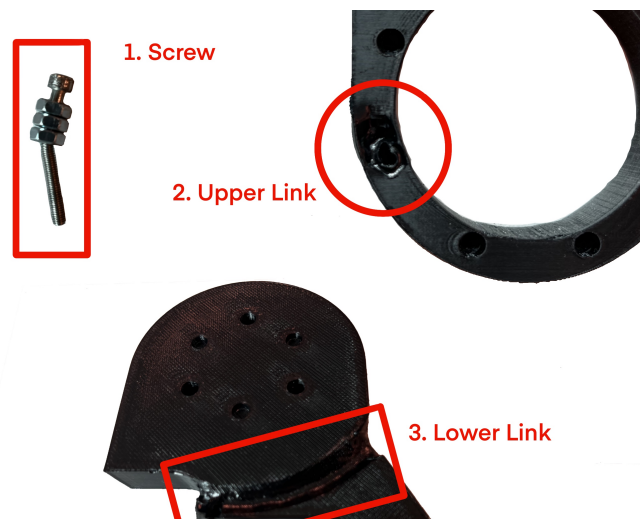
Figure 5.1: The result of aggressive testing of the actuator and physical stops during development.
