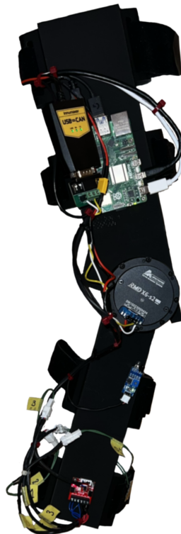
Figure 3.19: The final prototype of the Intelligent Knee Orthosis.
