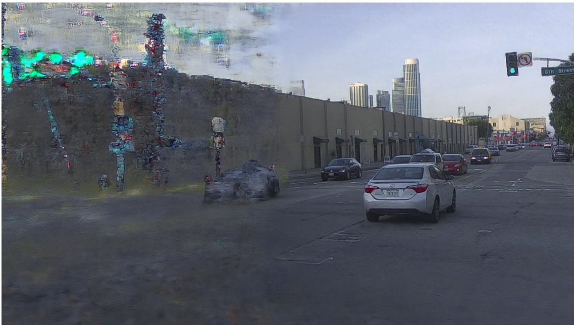
Figure 2.2: NeuRAD struggles to accurately render sections of the scene that were not observed during training. In this instance, the model is only trained with front-facing camera images. The figure shows the NeuRAD rendered image with the camera shifted 15 degrees to the left, thus illustrating the sharp quality difference between covered and non-covered sections.
