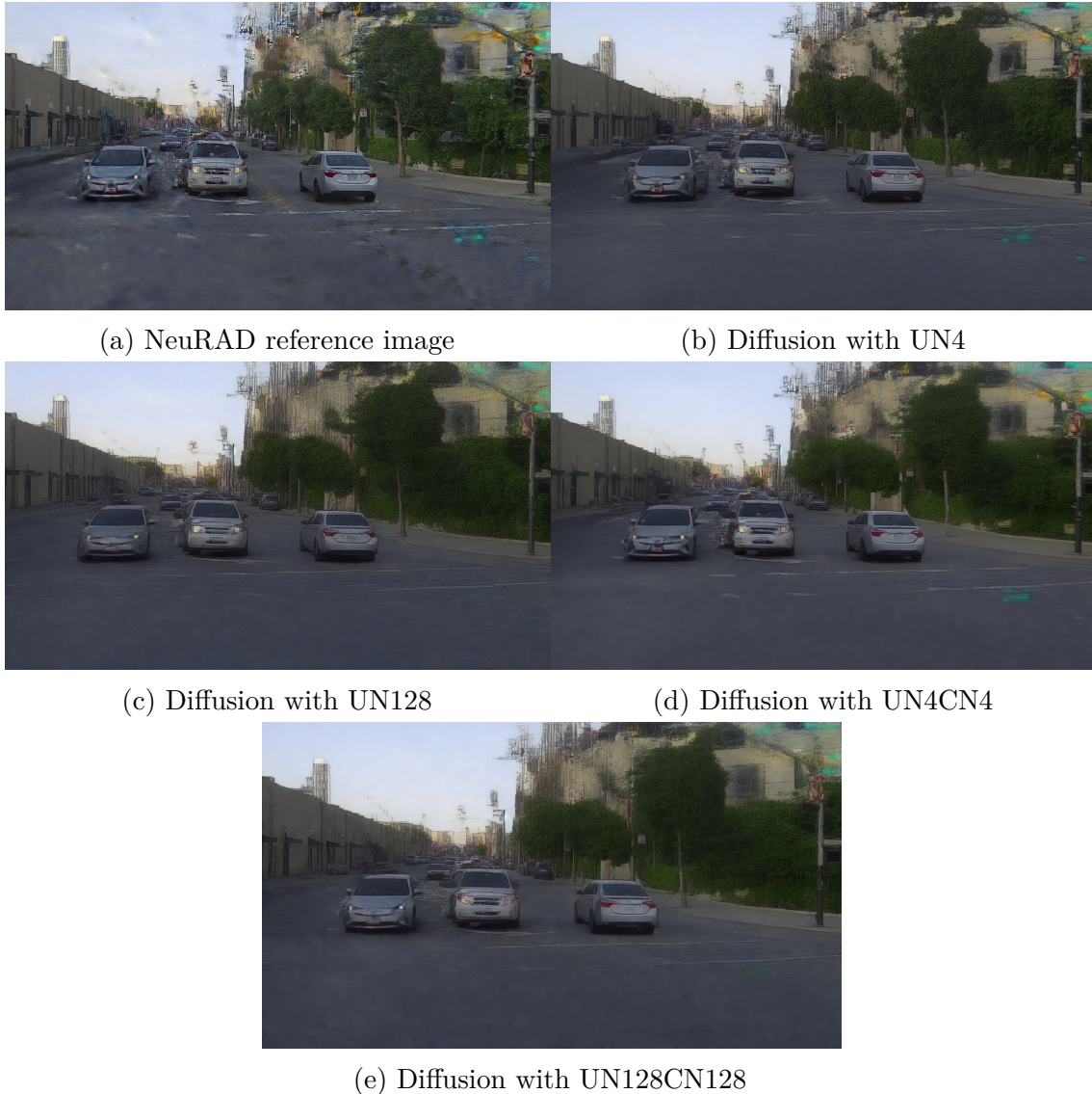
Figure 3.7: NeuRAD outputs which have been refined with Diffusion models finetuned with different configurations. (a) shows a poor NeuRAD render from a view in an area not covered in the training set. (b-c) show the image refined by a diffusion model which has been finetuned with LoRA rank 4 and 8 respectively, as mentioned in Section 3.4.2. (d-e) show the result of adding the ray as a conditioning signal, as outlined in Section 3.4.3.
