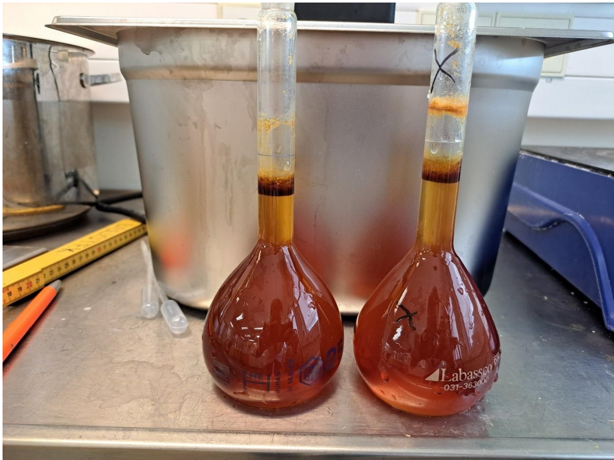
Figure 6. Early tests of soap separation, over a full day at 80°C. No difference in soap separation is visible.
