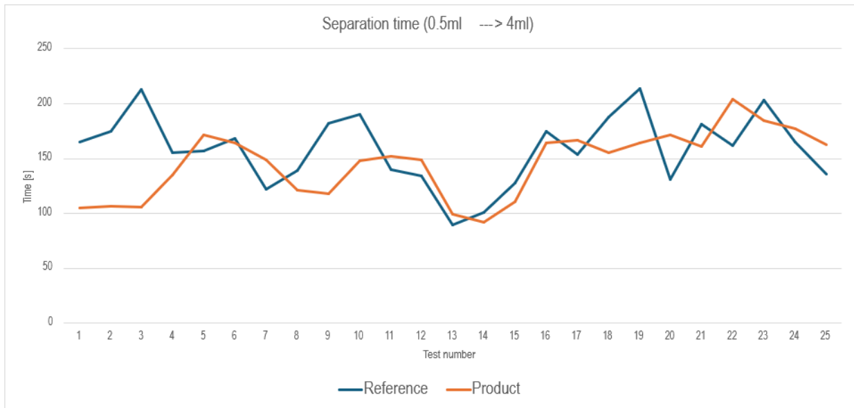
Figure 8. Results from the unoptimized speed test method.
