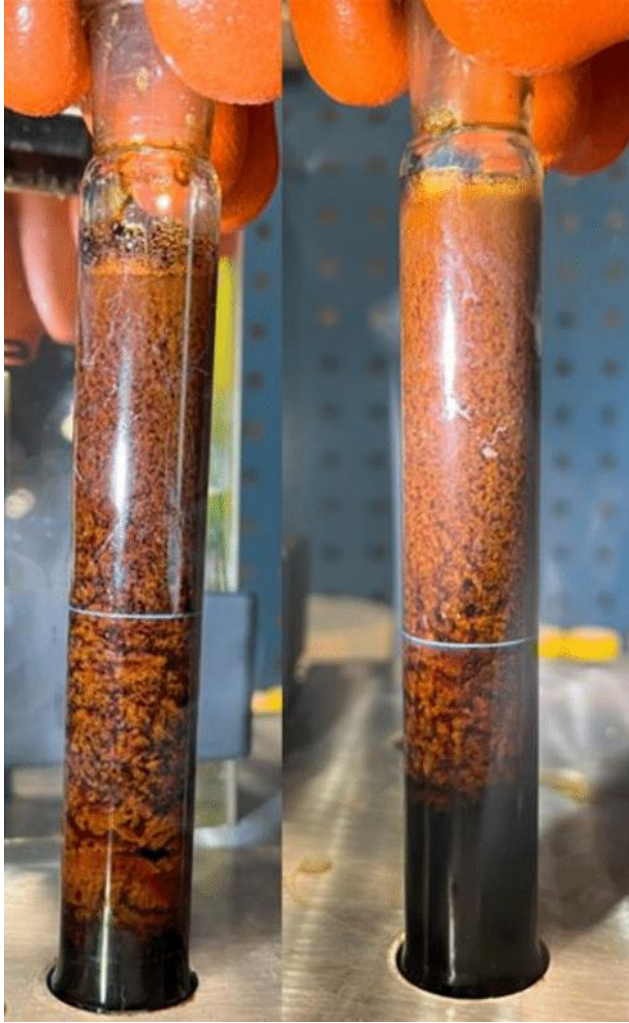
Figure 5. Tall oil soap separation in natural black liquor. Right test tube is treated with BIM's additives.
