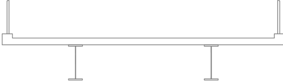
Figure 2.1: Conceptual design of a twin-girder cross section.
