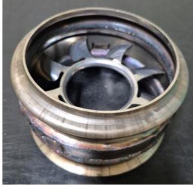
Figure 3.23 Mixer installed upstream of diffuser inlet
