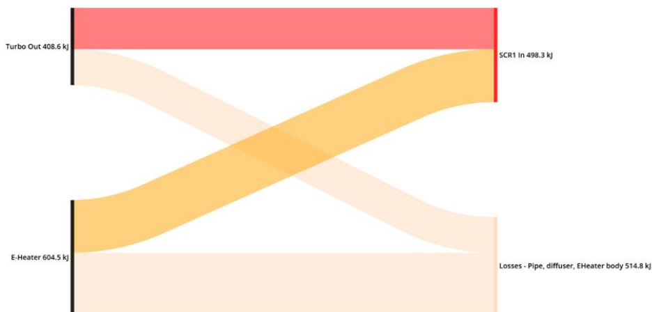
Figure 3.31 Energy flow between turbocharger outlet and SCR1 inlet for 74s of cold WHTC
