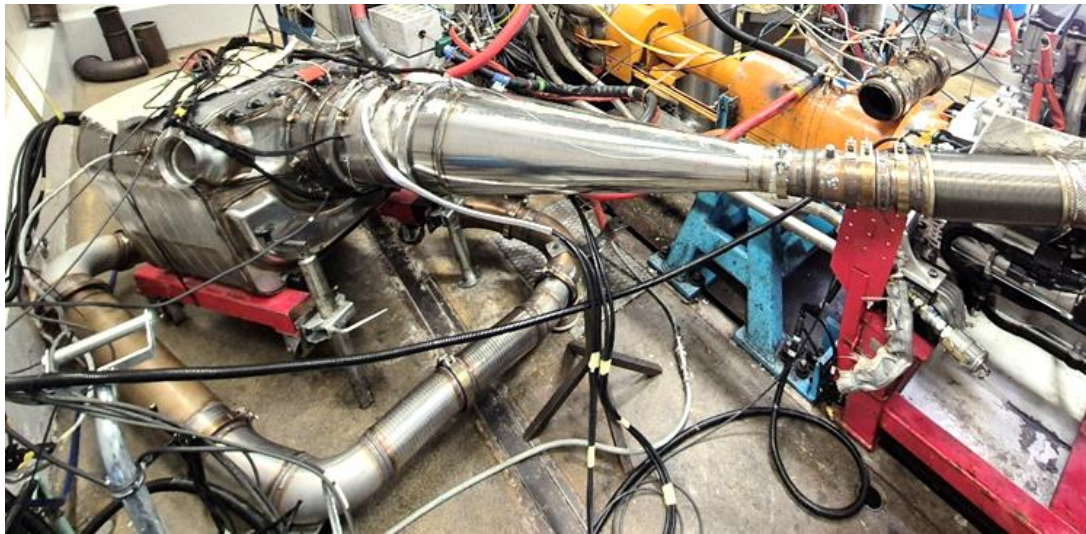
Figure 3.21 Silencer and heater installation in engine test rig
