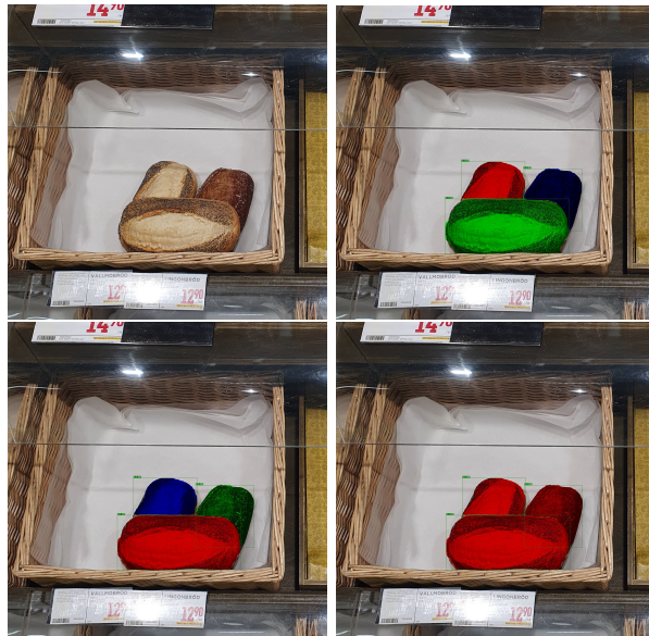
Figure 57: Results for clustering algorithms example 2, (top left) original image, (top right) DBSCAN result, (bottom left) Mean Shift result, (bottom right) Affinity Propagation result.
