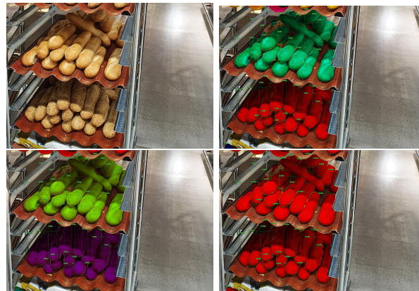
Figure 59: Results for clustering algorithms example 4, (top left) original image, (top right) DBSCAN result, (bottom left) Mean Shift result, (bottom right) Affinity Propagation result..
