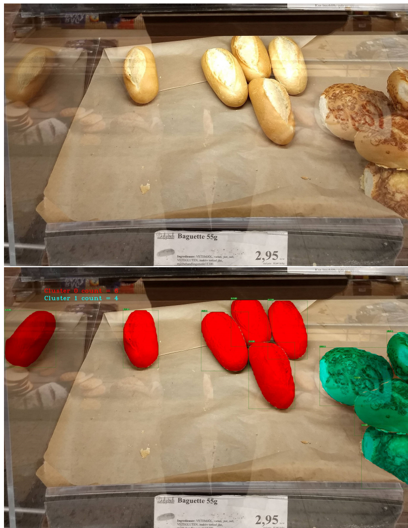
Figure 42: Input of the automatic inventory system (top); Output of the automatic inventory system (bottom).
