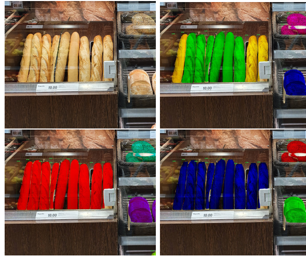
Figure 58: Results for clustering algorithms example 3, (top left) original image, (top right) DBSCAN result, (bottom left) Mean Shift result, (bottom right) Affinity Propagation result.
