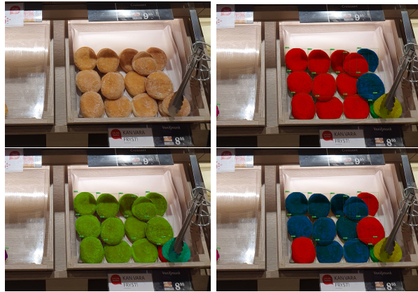
Figure 60: Results for clustering algorithms example 5, (top left) original image, (top right) DBSCAN result, (bottom left) Mean Shift result, (bottom right) Affinity Propagation result.
