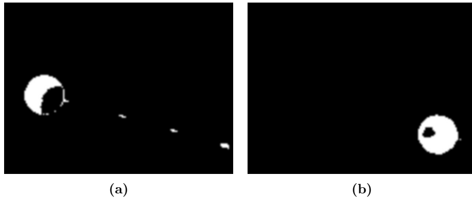
Figure 4.3: Problems with the background subtraction that occur even though the frames have been aligned perfectly. In 4.3a the object have become a part of the background model and in 4.3b the object passes over a patch of background with the same colour. The object is a yellow circle.
