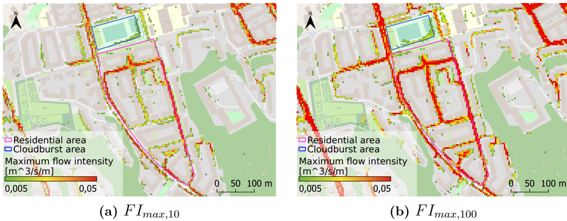
Figure 4.4: Maximum flow intensity during a (a) 10- and (b) 100-year rain (climate factor 1.2) in Säggatan. The legend describes the representation of residential and cloudburst areas. Also, the color scale is used to describe the flow intensities ( m^3/s/m ) from 0.005 (green) to 0.05 (red).
