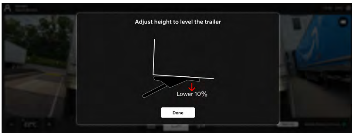
Figure 7.18: Adjust pop-up, helps user to adjust height of fifth wheel.
