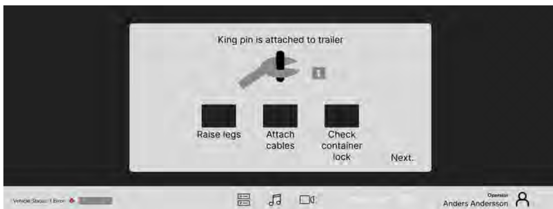
Figure 7.13: Wireframe of an example pop-up that reminds user to do routine checks.
