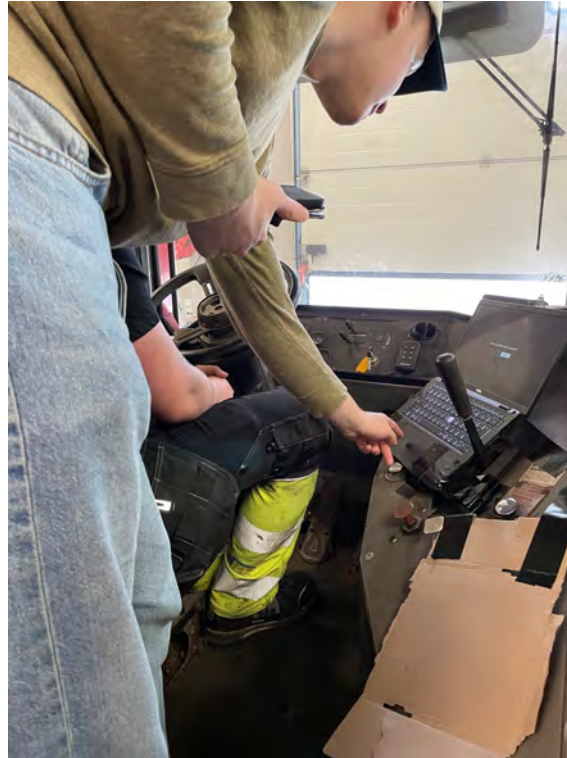
Figure 7.26: Image of a laptop set up within the terminal tractor as a test rig, demonstrating the integration of the interface for testing and evaluation purposes.
