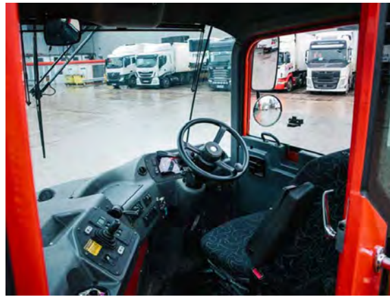
Figure 1.2: Existing cock-pit solution for a terminal tractor [6]. Copyright by Kalmar
