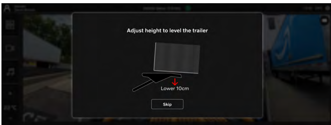
Figure 8.10: Final version of pop-up showcasing recommendations for fifth-wheel height adjustments.
