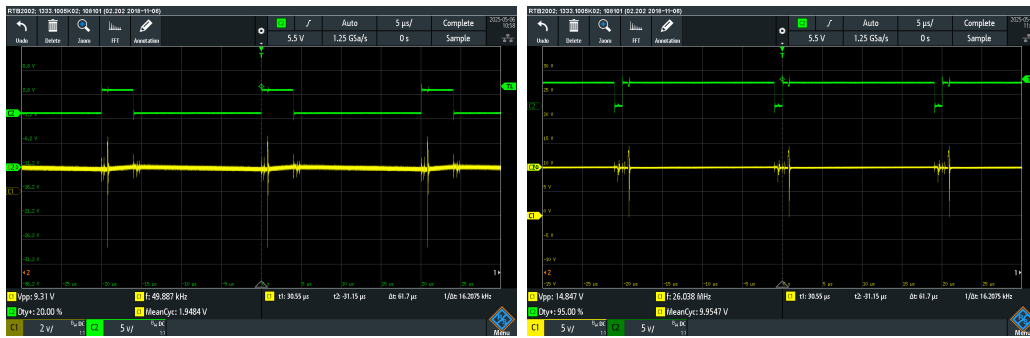
Figure 4.3: The green signal is a PWM sent from the Arduino with a duty percentage of 20% on the left image and a duty percentage of 95% on the right image. The yellow signals are the output voltage V_o of the buck with respect to the duty cycles. The left output voltage is around 2 V and the right output voltage is around 10 V
