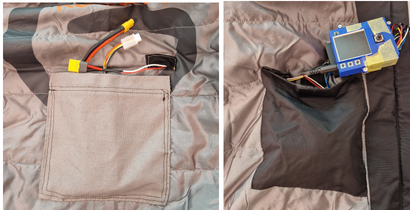
Figure 4.7: The battery pocket on the left picture, The user interface and buck pocket on the right picture
