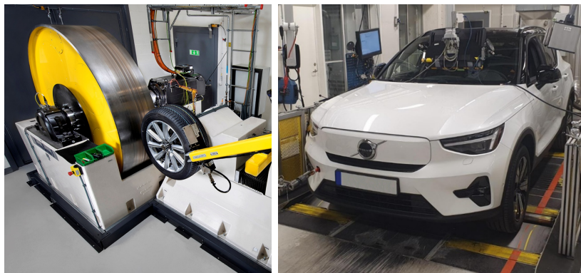
Figure 3.2: (L) Drum Test rig at PV16; (R) Dynamometer rig at EP (Images from Volvo Car Corporation Internal Media)
