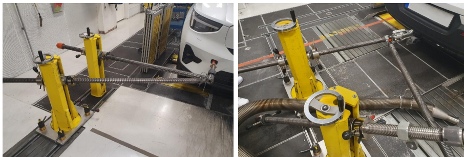
Figure 3.19: (L) Front Tow Point Mounting and (R) Rear Hitch Point Mounting (Images from Volvo Car Corporation Internal Media)
