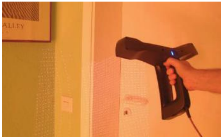
Figure 3: Data capturing with a 3D laser scanner (FARO Technologies, 2016a, pp. 7)
