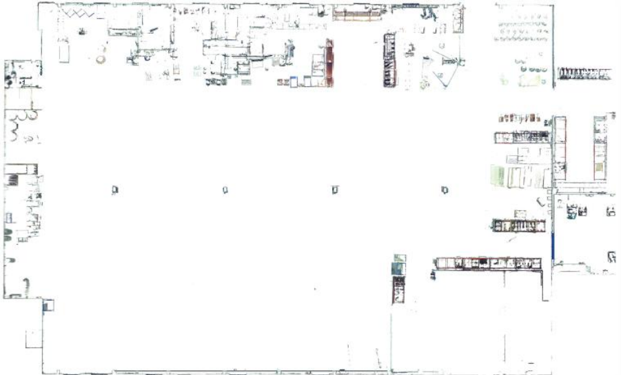
Figure 28: 2D-section of factory point cloud without floor
