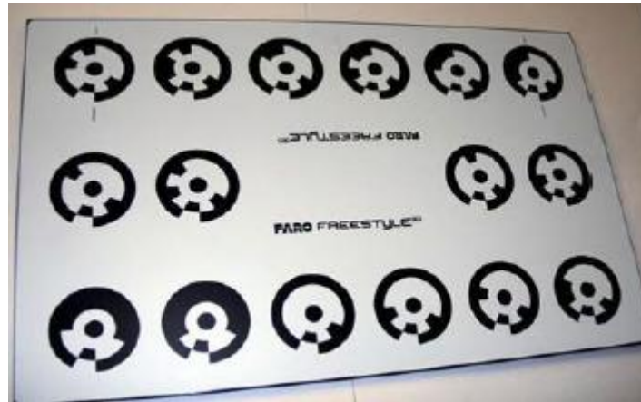
Figure 5: Calibration plate (FARO Technologies, 2016, pp. 89)
