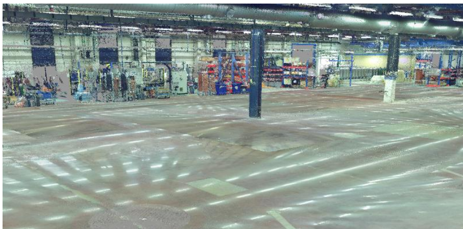
Figure 32: Unwanted stored objects removed from the factory point cloud
