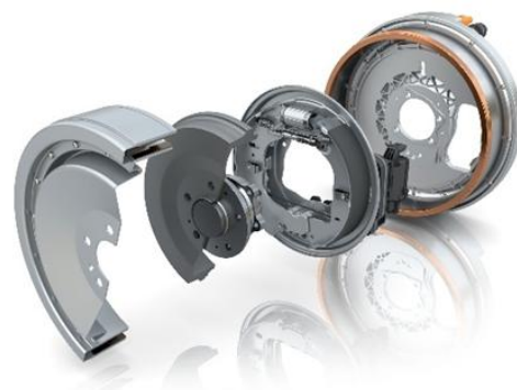
Fig. 14. Example of IWM integration concept from Continental [76]
