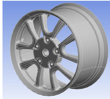
Fig. 63. Static Structural analysis geometry
