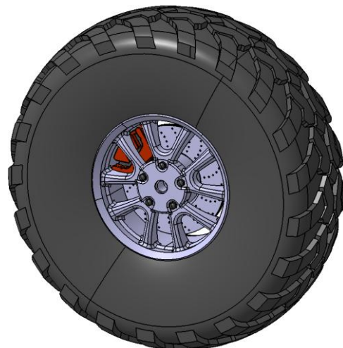
Fig. 39. Conventional wheel-end configuration with disc brake assembly
