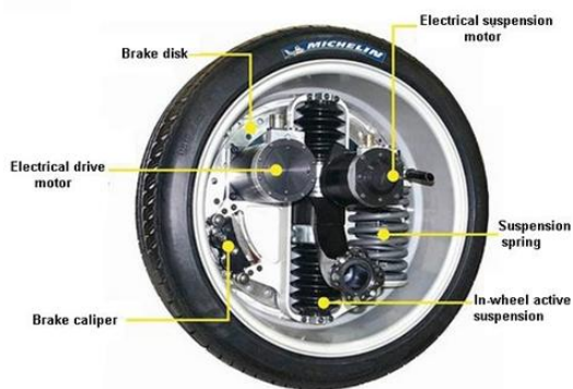
Fig. 15. Example of IWM integration concept from Michelin [75]
