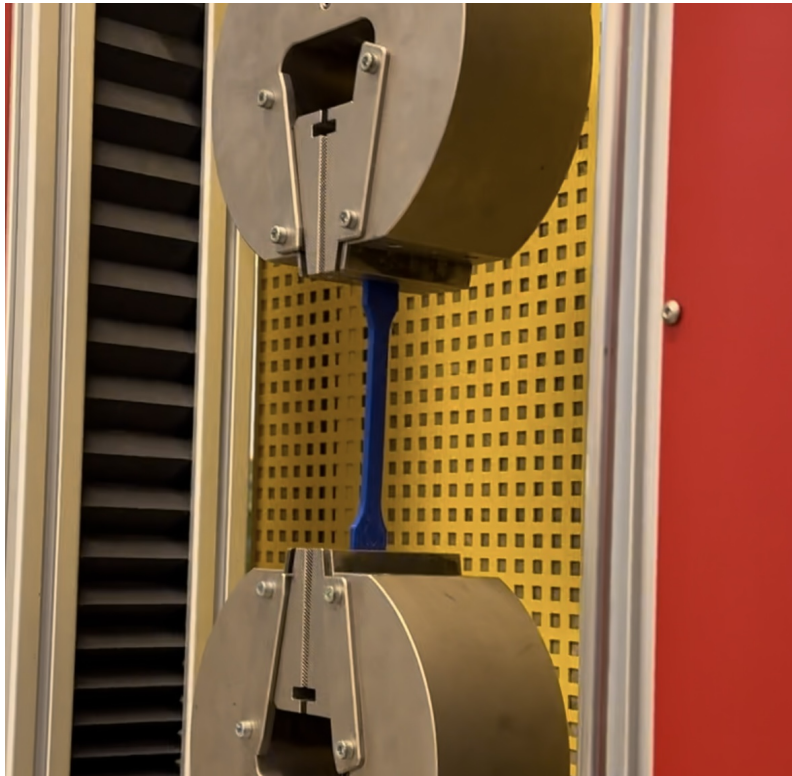
Figure 3.3: Test setup for 3D printed test specimens.
