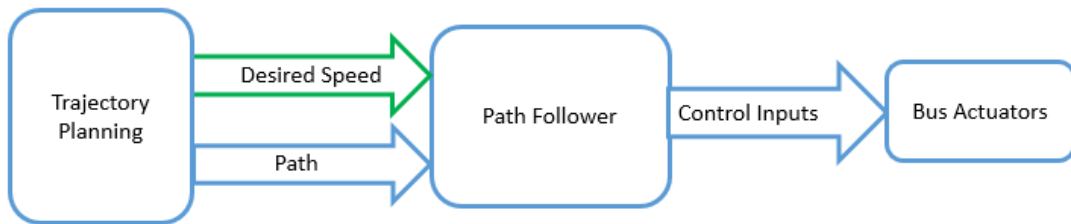
Figure 2.3: Path following controller: Input and output signals
