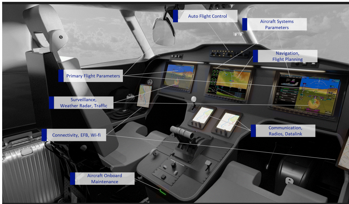
Figure 3.1: Illustration of ES-30 cockpit avionics suite.
