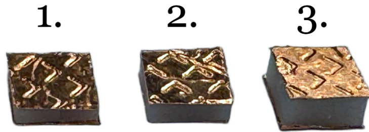
Figure 3.4: Sintered and HIPed additively manufactured cubes, with densities presented in Table 3.2. Note that copper tape is attached to them in this figure, which was done after the density measurements. The dimensions are given in Table 4.1.
