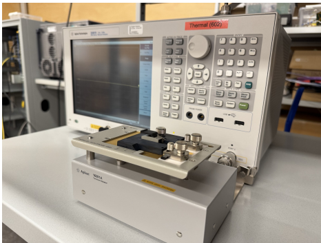
(a) Measurement setup for one-port S-parameter characterisation of a parallel plate capacitor.
