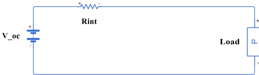
Figure 2.1: Simple R_{int} model
