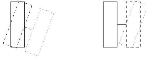
**Figure 4.1:** The kinematic interdependence when both the lateral displacement as well as the lateral creepage are achieved by one shaft. The rectangles represent wheel positions, where the solid rectangle is the original position, the dashed rectangle gives the position after the first motion and the dotted rectangle represents the final position.
