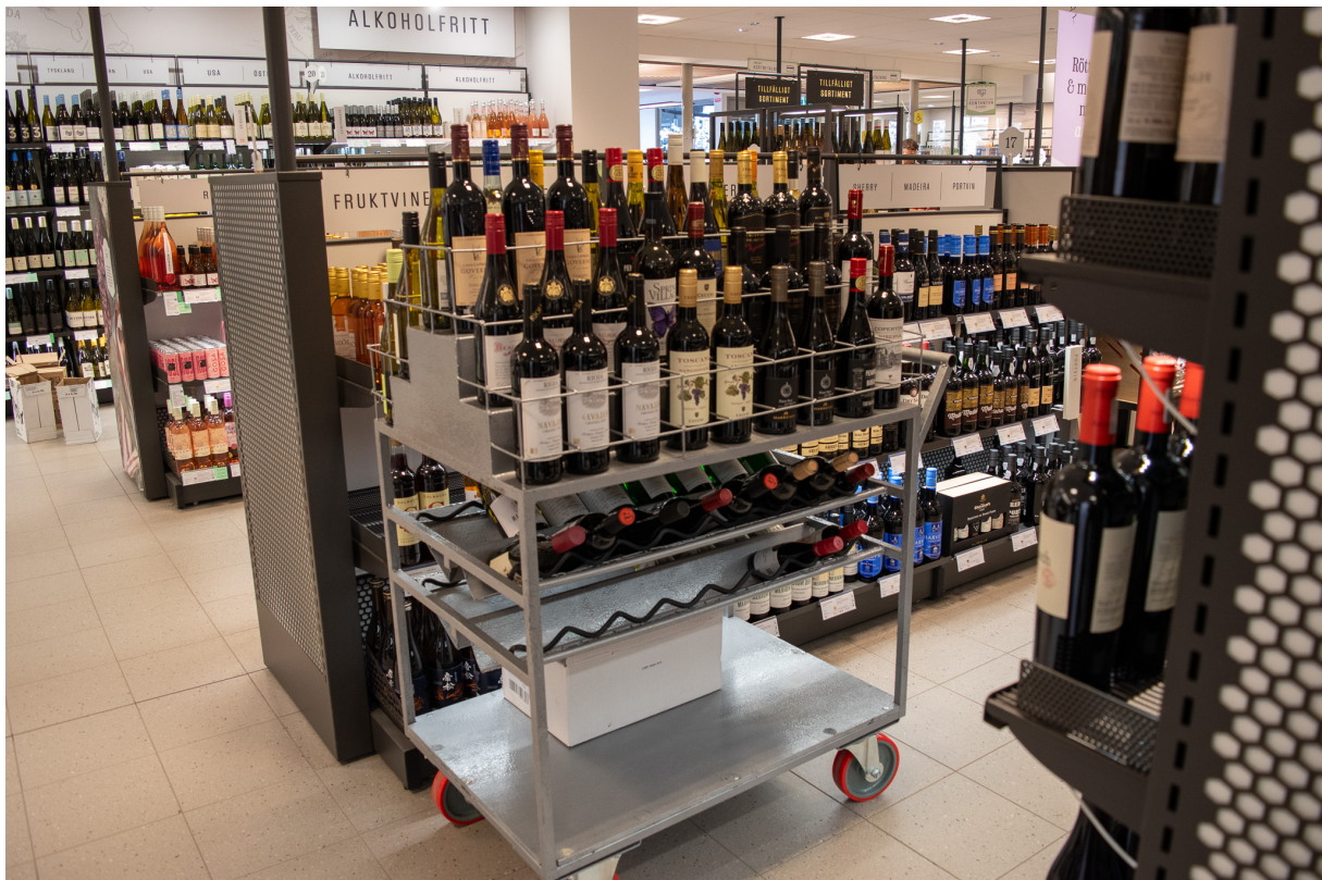
Final prototype of the Slattvagn, featuring the upper staircase structure (Trappan) and lower tilted slots.
