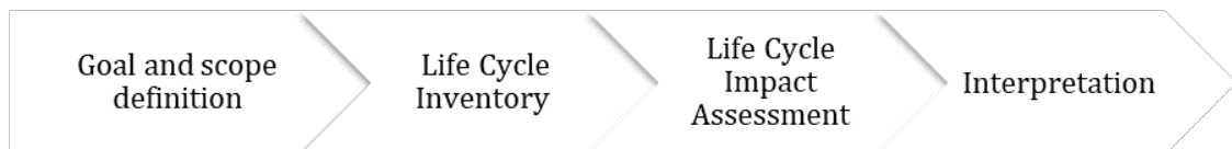
Figure 4.1: Stepwise methodology for performing a Life Cycle Analysis.
