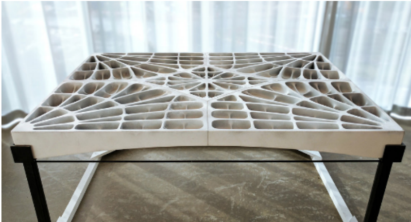
Figure 5.1: Climate optimized concrete “vault” structure developed by BRG (BRG, 2020).
