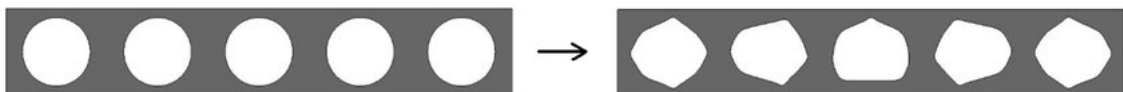
Figure 5.4: Illustration of shape optimization performed on a hollow core slab (Bendsøe & Sigmund, 2003).
