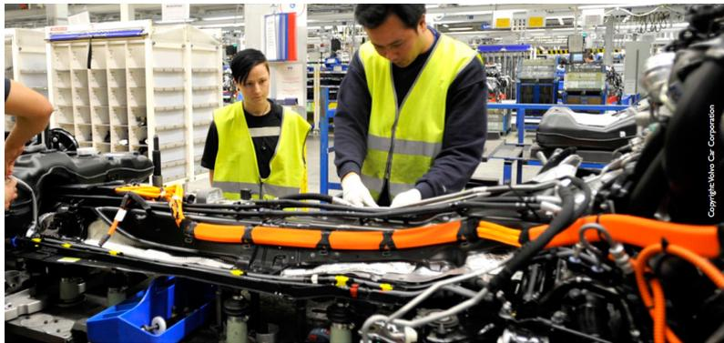
**Figure 1.1:** Installation of cable harnesses.
