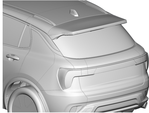
(b) Optimal design for minimising C_{LR} , while maintaining baseline levels of C_{DA} and C_{YM} .
