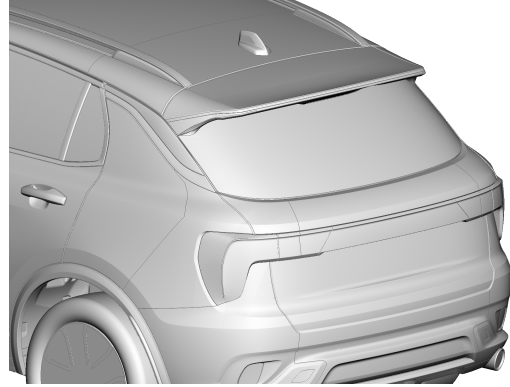
(b) Optimal design for minimising C_{YM} , while maintaining baseline levels of C_{DA} and C_{LR} .
