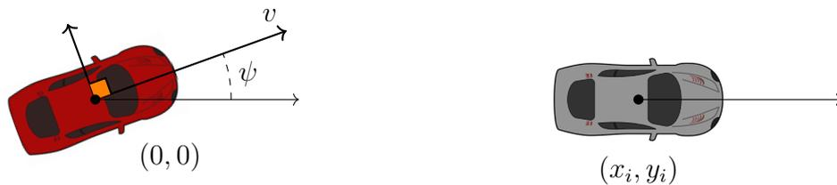
**Figure 3.2:** Top view of a single lane with ego vehicle (red) and a single vehicle (grey). Note that relative coordinates of surrounding objects,  $(x_k, y_k)$ , are given in the ego vehicle’s body frame, where the  $x$ -axis is along the forward direction of the ego vehicle and the  $y$ -axis perpendicular to it in a right-handed coordinate system.
