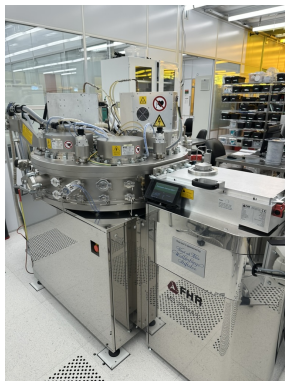
Figure 3.4: The FHR MS 150x4-L magnetron sputtering system used for TiN deposition.
