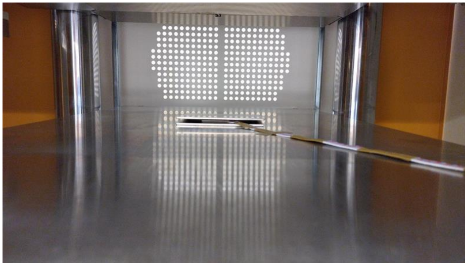
Figure 20: Internal temperature measurement during a decal transfer.
