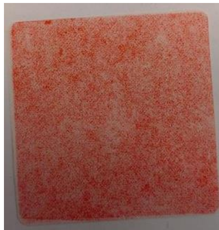
Figure 19: Pressure distribution in the hot press for a 33 cm 2 sample.
