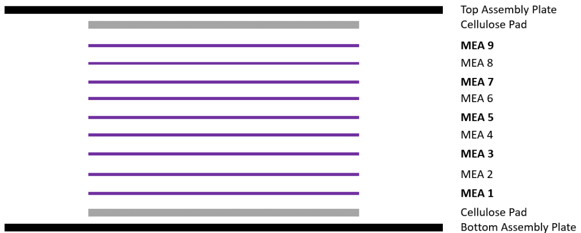
Figure 38: Experimental setup of the MEAs in the series stacking experiment for in-situ performance testing.
