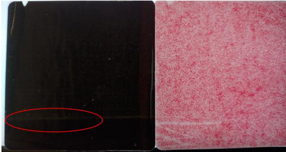
Figure 24: Localized electrode defects appear on the pressure film.
