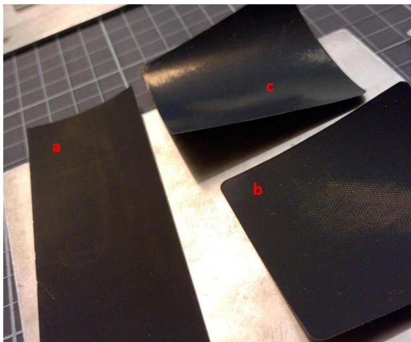
Figure 26: Reflexion behavior for (a) the raw electrode, (b) the p0 annealed electrode and (c) the p300 annealed electrode.
