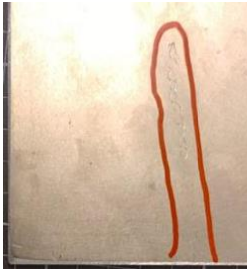
Figure 15: Assembly plate damaged instead of the hot press.
