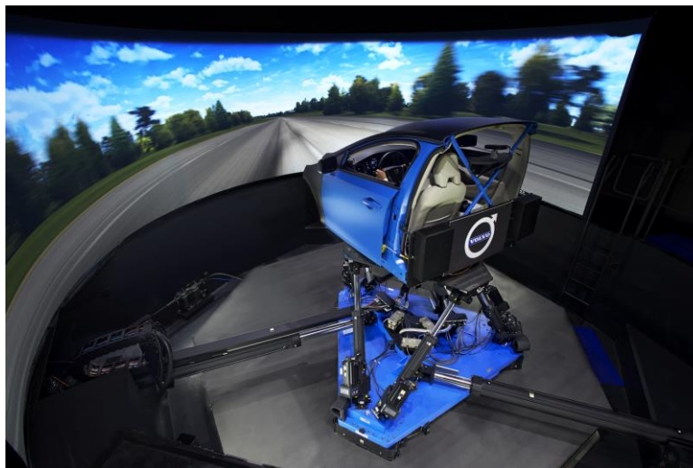
Figure 14: Vehicle Dynamics simulator at Volvo Car Corporation [15]
